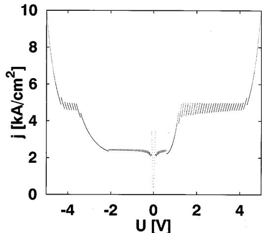
FIG. 1. Simulated current–voltage characteristic of a superlattice with 40 periods and  $N_D=6.7\times 10^{17}$  cm<sup>-3</sup> (sweep-up). The 32nd barrier of the superlattice has been chosen 20% wider than the others.
