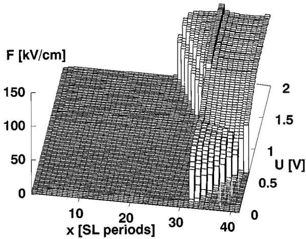
FIG. 2. Simulated spatial profiles of the electric field  $F$  across the superlattice (SL) structure for positive voltages (Fig. 1). The SL periods are numbered starting from the cathode.
