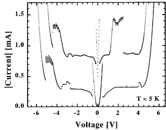
FIG. 3. Measured current–voltage characteristics in the dark (lower curve) and under illumination (upper curve) of a GaAs/AlAs superlattice with an intentional substantial increase of the thickness of one AlAs barrier layer. For both bias directions the absolute value of the current for the sweep-up direction is displayed. The upper curve is vertically shifted by 0.5 mA.
