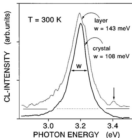
FIG. 4. Cathodoluminescence spectra of a *c*-GaN crystal (sample B) and of a *c*-GaN layer (sample D) at 300 K. The arrow at about 3.4 eV marks the contribution from inclusions of *h*-GaN in the layer.
