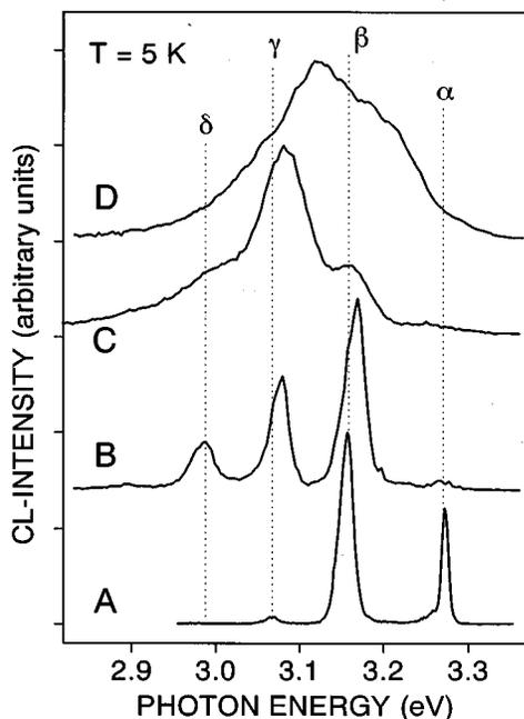
FIG. 2. Cathodoluminescence spectra of *c*-GaN crystals and layers. Spectra A to D correspond to the respective samples described in the text.
