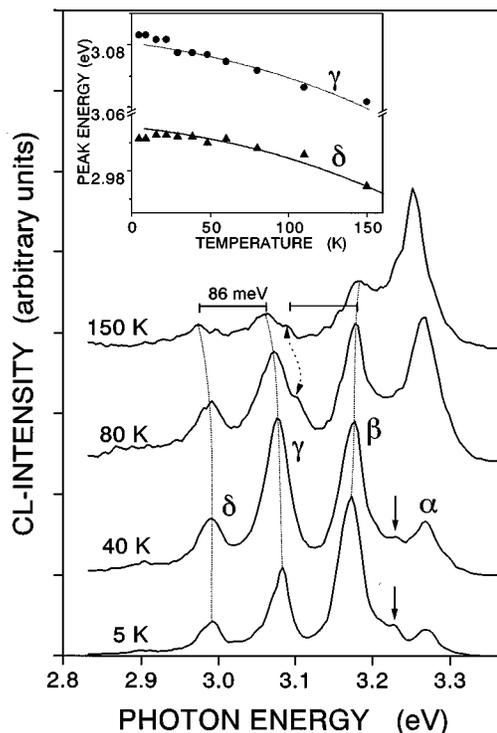
FIG. 3. Cathodoluminescence spectra of *c*-GaN crystals (sample B) at different temperatures. The bars mark the energy spacing of the phonon replica in *c*-GaN.<sup>6</sup> Inset: Temperature dependence of the peak energy of the CL lines  $\delta$  and  $\gamma$ . The solid lines mark the rigidly shifted temperature dependence of the band-gap energy of *c*-GaN according to Ref. 12.
