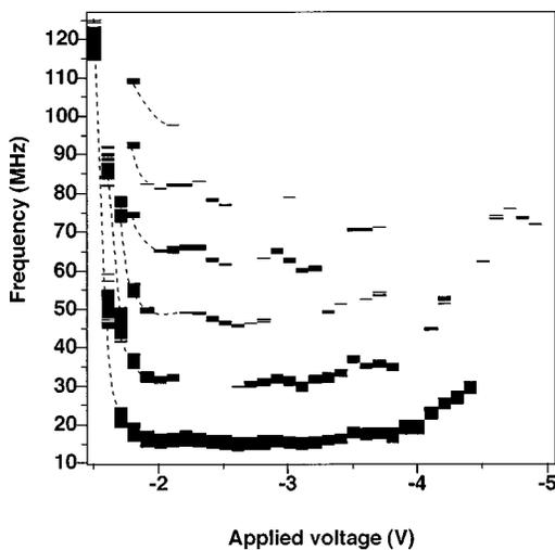
FIG. 2. Power spectra of self-oscillations vs applied voltage for a laser intensity of  $2$  mW at  $20$  K. Black areas correspond to large amplitudes. The dashed lines have been added as a guide to the eye.
