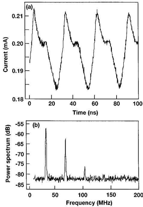
FIG. 1. (a) Current self-oscillations and (b) corresponding power spectrum at  $-3$  V for a laser intensity of  $2.5$  mW at  $20$  K.
