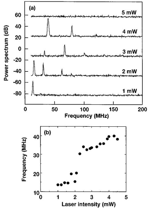
FIG. 3. (a) Power spectra of self-oscillations for  $-3$  V for different laser intensities between  $1$  and  $5$  mW at  $20$  K. The different spectra have been shifted by  $35$  dB with respect to each other in order not to overlap. (b) Fundamental frequency vs laser intensity for  $-3$  V at  $20$  K.
