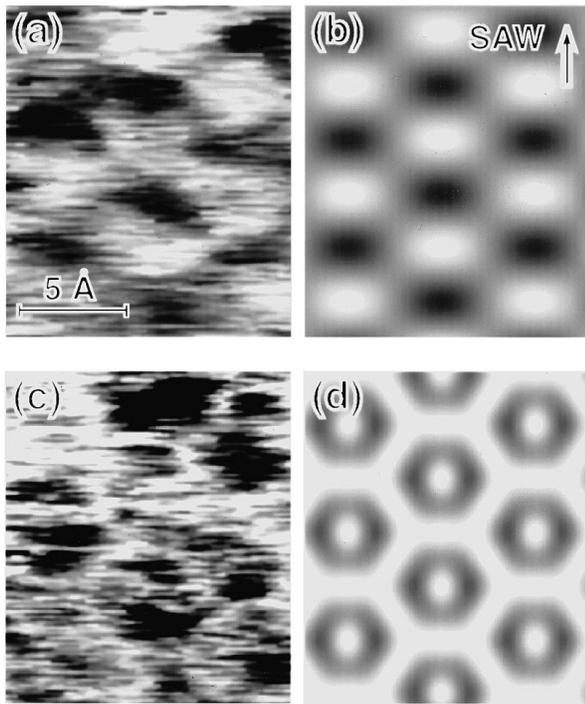
FIG. 2. Comparison of the measured (a) and (c) with the modeled (b) and (d) phase and amplitude, respectively, showing atomic resolution. The arrow in (a) indicates the SAW propagation direction.
