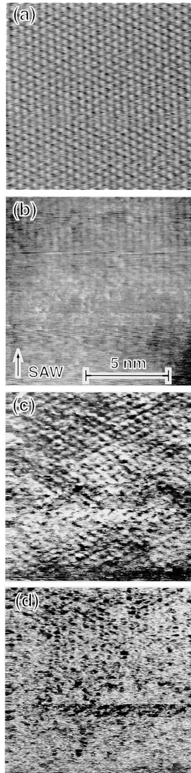
FIG. 1. Undisturbed topography image of the hexagonal Au(111) surface measured by STM (a). Topography showing reduced contrast (b), atom-resolved phase (c), and amplitude (d) measured simultaneously by SATM.
