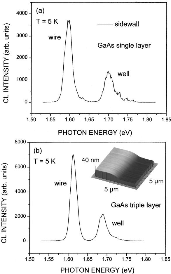
FIG. 4. CL spectra at 5 K excited at the fast growing sidewall of (a) the single and (b) the stacked multiple lateral quantum-wire structure on patterned GaAs (311)A substrates. The nominal GaAs layer thickness is 2 nm. The inset shows the three-dimensional AFM image of the 15-nm-high sidewall of the multiple quantum-wire structure.
