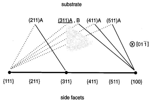
FIG. 2. Schematic diagram of the facets formed during growth on patterned GaAs (211)A, (311)A&B, (411)A, and (511)A substrates for mesa stripes along  $[01-1]$ . The upper line denotes the orientation of the substrate surfaces and the lower one the orientation of the facets determined from the AFM measurements in Fig. 1. The dashed lines point toward the sidewalls observed on the left-hand side from Fig. 1 and the solid lines point toward those of the right-hand side.
