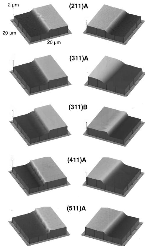
FIG. 1. Three-dimensional AFM images of the edges of the 400-nm-high mesa stripes along  $[01-1]$  after overgrowth on GaAs (211)A, (311)A, (311)B, (411)A, and (511)A substrates. The scanning area is  $20 \times 20 \mu\text{m}^2$ , and the full scale in height is  $2 \mu\text{m}$ .
