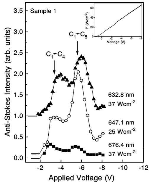
FIG. 2. Voltage dependence of anti-Stokes LO-phonon intensity of sample 1 at 5 K. The arrows label the  $C_1 \rightarrow C_4$  and  $C_1 \rightarrow C_5$  tunneling resonances. Three excitation wavelengths are used. Inset: Voltage dependence of the electrical power input of the same sample using an excitation density of  $37 \text{ W cm}^{-2}$  at 632.8 nm.
