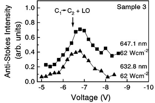
FIG. 4. Voltage dependence of the anti-Stokes LO-phonon intensity of sample 3 at 5 K. The Raman signal peaks at the voltage where  $C_1 \rightarrow C_2 + \text{LO}$  resonant tunneling occurs. Two excitation wavelengths are used.
