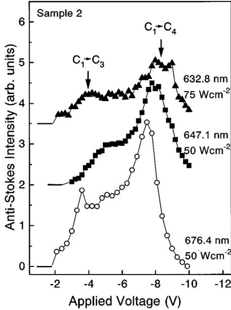
FIG. 3. Voltage dependence of the anti-Stokes LO-phonon intensity of sample 2 at 5 K. The arrows label the  $C_1 \rightarrow C_3$  and  $C_1 \rightarrow C_4$  tunneling resonances. Three excitation wavelengths are used.
