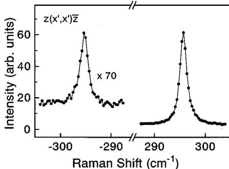
FIG. 1. Typical Stokes and anti-Stokes Raman spectra of sample 1 at 5 K for an applied voltage of  $-6 \text{ V}$  using an excitation density of  $37 \text{ W cm}^{-2}$  at 632.8 nm.
