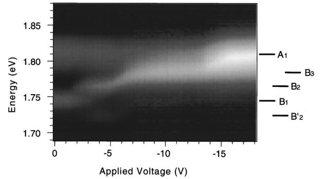
FIG. 5. PL spectra as a function of the negative bias at 20 K for a laser intensity of 1 mW. The PL intensity is indicated on a gray scale, where a large intensity corresponds to a bright region.
