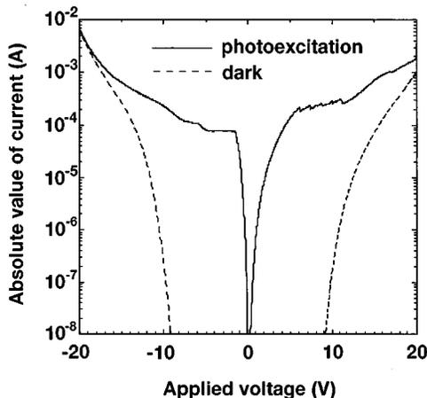
FIG. 2.  $I$ - $V$  characteristics in the dark and for a laser intensity of  $1$  mW at  $20$  K. A positive voltage corresponds to a positive bias applied to the  $n^+$ -GaAs substrate.
