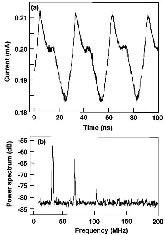
FIG. 3. Time-resolved photocurrent at  $-3$  V (a) and corresponding power spectrum (b) at  $20$  K for a laser intensity of  $2.5$  mW.
