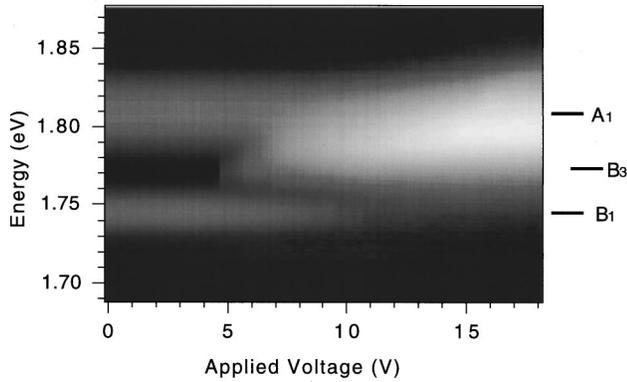
FIG. 4. PL spectra as a function of the positive bias at 20 K for a laser intensity of 1 mW. The PL intensity is indicated on a gray scale, where a large intensity corresponds to a bright region.
