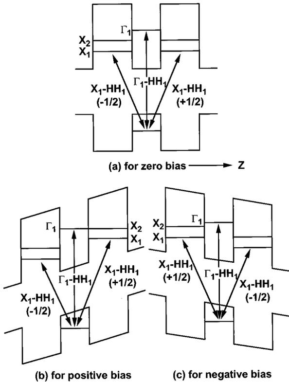
FIG. 1. Schematic diagram of the energy level structure in the conduction band of the investigated type-II GaAs-AlAs superlattice (a) at zero bias, (b) at positive bias for resonant transfer from  $X_2$  to  $\Gamma_1$ , and (c) at negative bias for resonant tunneling from  $X_1$  to  $X_2$ .
