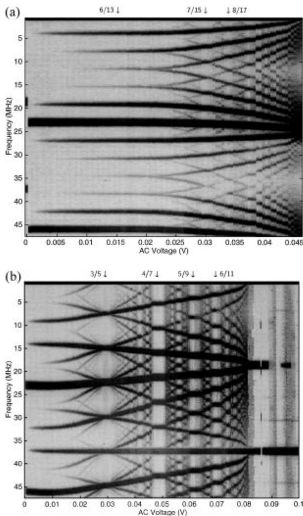
FIG. 2. Frequency bifurcation diagrams for a driving frequency of 50.0 (a) and 37.5 MHz (b) at 4.2 K. The logarithmic current power spectra are shown as a density plot vs the driving voltage. Darker areas correspond to larger amplitudes. The winding numbers are indicated above each graph.
