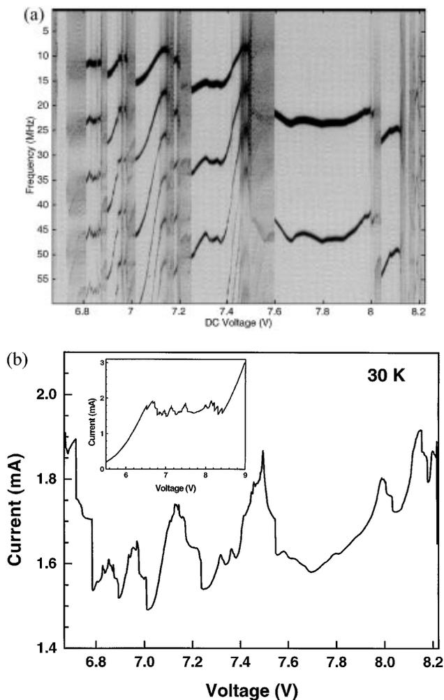
FIG. 1. (a) Frequency spectra of spontaneous current oscillations vs applied voltage at 30 K. The current power spectra are shown as a density plot on a logarithmic scale, where darker areas correspond to larger amplitudes. (b) Time-averaged  $I$ - $V$  characteristic at 30 K with the inset showing the whole plateau.
