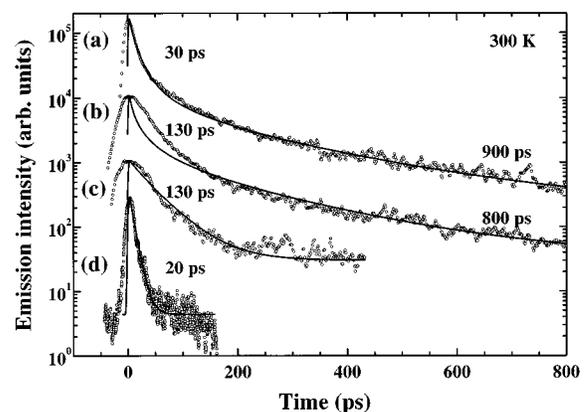
FIG. 1. Transients of the surface emission (symbols) in backscattering geometry at 300 K. The excitation fluences are 12, 3, 0.1, and  $0.01 \mu\text{J cm}^{-2}$  for transients (a), (b), (c), and (d), respectively. The traces are vertically shifted for clarity. The solid lines are fits of a recombination model. The major decay times are indicated.
