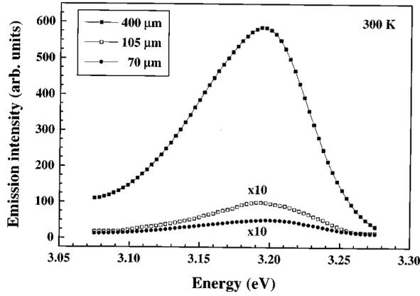
FIG. 2. Edge emission spectra for different excitation stripe lengths for a fluence of  $20 \mu\text{J cm}^{-2}$  at 300 K.
