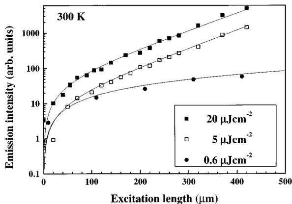
FIG. 3. Total edge emission vs excitation stripe length for different fluences at 300 K. The lines are fits of model calculations to deduce the respective gain values.
