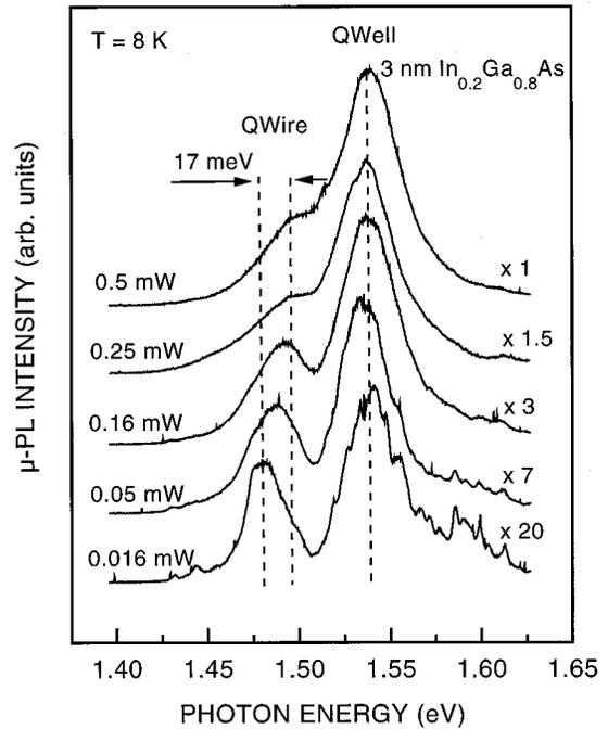
FIG. 2.  $\mu\text{-PL}$  spectra taken at 8 K excited on the (InGa)As wire region connected with the 3-nm-thick  $\text{In}_{0.2}\text{Ga}_{0.8}\text{As}$  quantum well for different excitation power.
