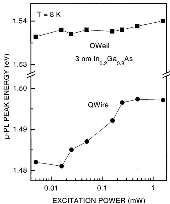
FIG. 3.  $\mu$ -PL peak energy positions at 8 K of the (InGa)As quantum wire and quantum well in dependence on the excitation power. The thickness of the quantum well is 3 nm with an In composition of 0.2.
