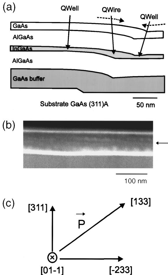
FIG. 1. (a) Schematic of the strained (InGa)As sidewall quantum wire on patterned GaAs (311)A substrates and (b) cross-sectional SEM image of the (InGa)As quantum wire connected with the 6-nm-thick  $\text{In}_{0.2}\text{Ga}_{0.8}\text{As}$  quantum well (see arrow). In (c), the vector of the piezoelectric polarization in the strained wire is indicated.
