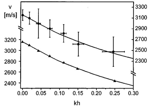
FIG. 5. SAW phase velocity dispersion  $v(kh)$  of Au covered ST-X quartz with  $k$  being the wave vector and  $h$  the Au layer thickness. The velocity was measured for seven values of  $kh$  over a lateral distance of ( $\circ$ )  $200$  nm and ( $\triangle$ )  $10\pi$  phase delay ( $28.3 - 36.0 \mu\text{m}$ ). The solid lines represent the calculated dispersion curve.
