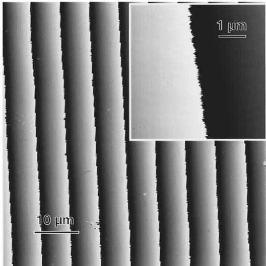
FIG. 2. SAFM measurement of the linear phase behavior of the plane waves excited by interdigital transducers. The phase jumps induced by the lock-in phase range of  $360^\circ$  have a separation of  $6.83 \mu\text{m}$ . The inset zooms on such a phase jump demonstrating the stability of the phase measurement.
