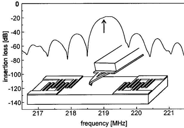
FIG. 1. Amplitude-frequency characteristic of the acoustic delay line formed by two interdigital transducers. The arrow marks the driving frequency. The inset shows the experimental setup.
