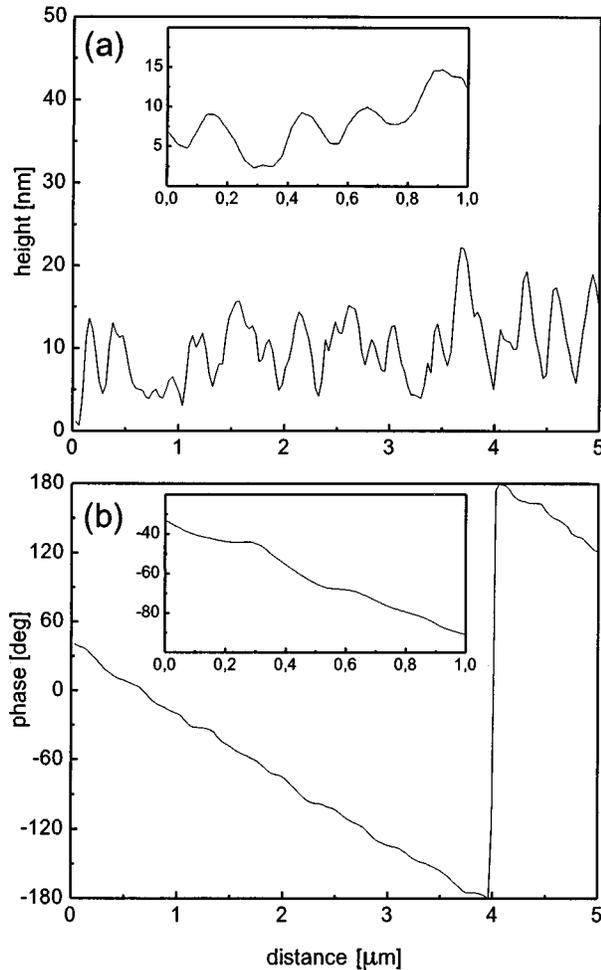
FIG. 4. SAFM measurement of (a) topography and (b) phase of a rough Au layer. The insets show the influence of the topographical gradients on the phase measurement.
