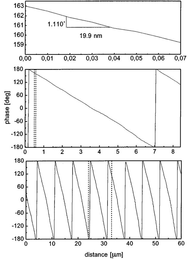
FIG. 3. Line scans of the linear phase dependence measured by the SAFM with the lower trace showing the  $60 \mu\text{m}$ , the middle trace the  $8.4 \mu\text{m}$ , and the upper trace the  $70 \text{ nm}$  measurement. The dotted lines mark the zooming in from the lower to the upper trace. For small scale scans the phase velocity is determined by the estimation of the phase slope. The maximum lateral resolution of the phase velocity determination was  $19.9 \text{ nm}$ .
