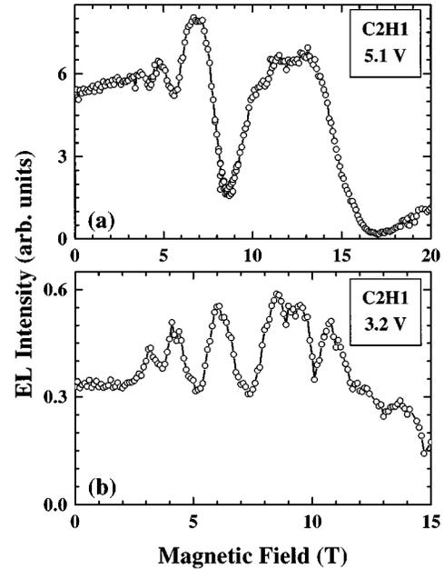
FIG. 2. Electroluminescence intensity of the  $C2H1$  interband transition in sample 1 (a) and sample 2 (b) as a function of the applied magnetic field at 5 K. The applied voltage was adjusted to the corresponding  $C2 \rightarrow C1$  resonance value (5.1 V in sample 1 and 3.2 V in sample 2).
