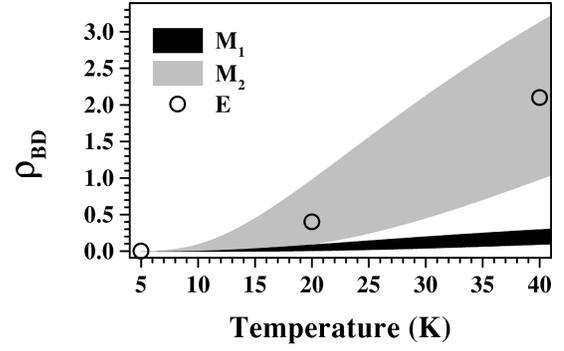
FIG. 3.  $M_1$ : possible values for  $\rho_{BD}$  according to Eq. (11),  $M_2$ : possible values for  $\rho_{BD}$  taking into account the areal densities  $a_B$  and  $a_D$ , and E: the experimental results for  $\rho_{BD}$  as a function of the temperature.
