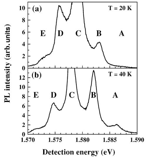
FIG. 2. PL spectra for resonant excitation into island C at (a) 20 and (b) 40 K. The integrated intensity ratio of peaks B and D has a value of about 0.4 and 2.1 at 20 and 40 K, respectively.
