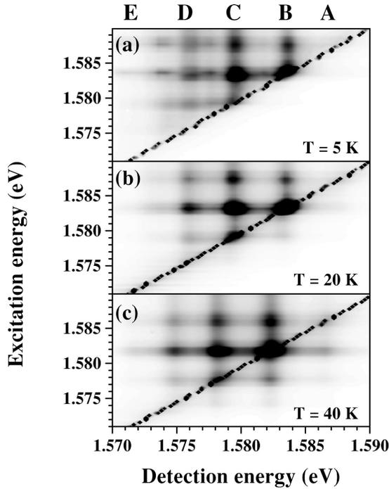
FIG. 1. PL intensity of a 5.5-nm-wide QW as a function of detection as well as excitation energy at (a) 5, (b) 20, and (c) 40 K. The PL spectra exhibit PL maxima for 5 monolayer islands A–E (marked on top). The images are divided by the laser energy (dotted line) into the Stokes region, i.e., where  $E_{\text{det}} < E_{\text{exc}}$  (upper-left part), and the anti-Stokes region, i.e.,  $E_{\text{det}} > E_{\text{exc}}$  (lower-right part).
