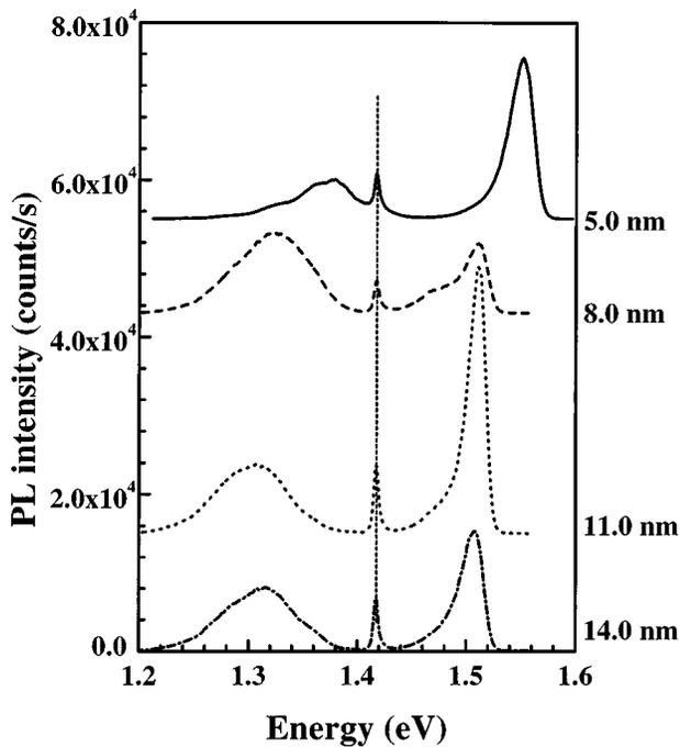
FIG. 2. Steady-state photoluminescence spectra of all four InAlAs/AlAsSb samples for a temperature between 7 and 10 K, excitation energy of 1.676 eV, and laser power of 50  $\mu$ W. The different samples are labeled by their respective InAlAs layer thickness. The vertical line marks the position of the InP:Fe substrate peak. The spectra for the 11.0, 8.0, and 5.0 nm samples have been vertically shifted by  $1.5 \times 10^4$ ,  $4.3 \times 10^4$ , and  $5.5 \times 10^4$  counts/s, respectively.
