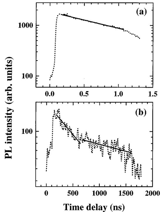
FIG. 4. Photoluminescence transients of the InAlAs buffer layer (a) and the MQW structure with 8.0 nm InAlAs (b) for a temperature of 6 K detected at 1.51 and 1.32 eV, respectively. Note the very different time scales in (a) and (b). The solid lines indicate linear fits corresponding to exponential decay times with values of 0.86 and 3.9  $\mu$ s.
