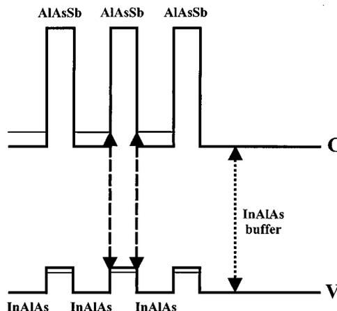
FIG. 1. Schematic diagram of the type II band alignment in InAlAs/AlAsSb multiple quantum well structures. The letters C and V indicate the edge of the conduction and valence band, respectively. The vertical arrows indicate the spatially indirect recombination at the InAlAs/AlAsSb heterointerfaces and the direct recombination in the InAlAs buffer layer.
