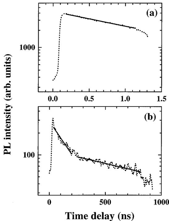
FIG. 3. Photoluminescence transients of the InAlAs buffer layer (a) and the MQW structure with 5.0 nm InAlAs (b) for a temperature of 6 K detected at 1.55 and 1.38 eV, respectively. Note the very different time scales in (a) and (b). The solid lines indicate linear fits corresponding to exponential decay times with values of 0.19 and 1.2  $\mu$ s.
