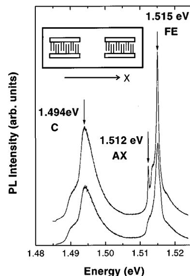
FIG. 1. GaAs photoluminescence without (upper curve) and under the influence of a surface acoustic wave (lower curve), recorded with an excitation wavelength  $\lambda_L=514.5 \text{ nm}$ . The spectra are displaced vertically. The inset shows the configuration of the transducers.
