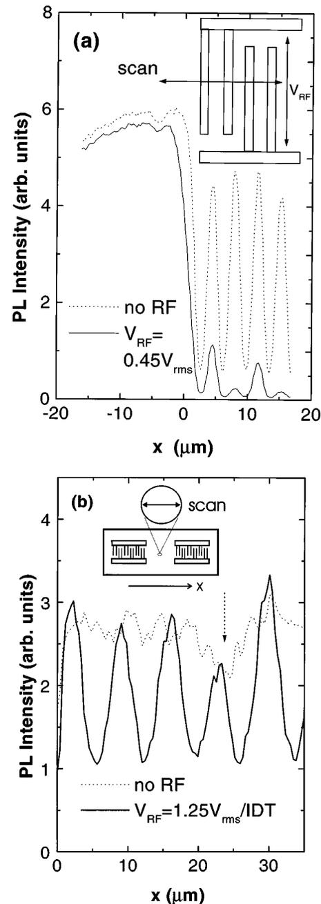
FIG. 3. (a) Free-exciton luminescence profiles (emission at 1.515 eV) close to the edge of the IDT and (b) under a standing wave between the IDT's. The solid and dashed lines display the corresponding profiles for powered and unpowered IDT's, respectively. The insets show the corresponding scan regions.
