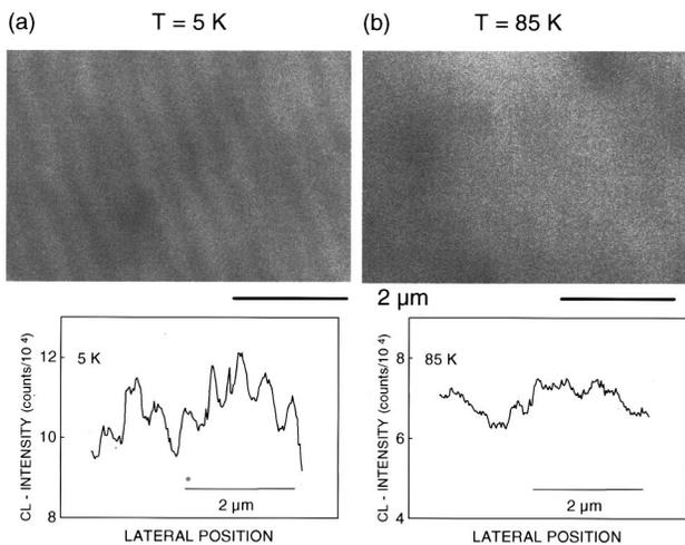
FIG. 3. Lateral CL-intensity distribution detected at the quantum wire peak position (a) at 5 K (1.611 eV) and (b) at 85 K (1.604 eV) together with the corresponding CL-intensity linescans across the wires.
