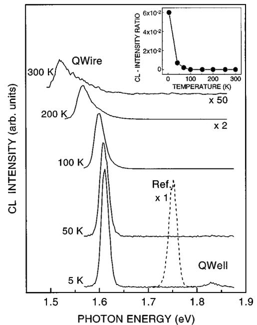
FIG. 2. CL spectra of the sidewall quantum-wire array on patterned GaAs (311)A substrates between 5 K and room temperature (solid lines) and of the reference quantum-well sample on the planar substrate (dashed line). The inset shows the ratio of the CL intensity from the connecting quantum wells to that of the sidewall quantum wires as a function of the temperature.
