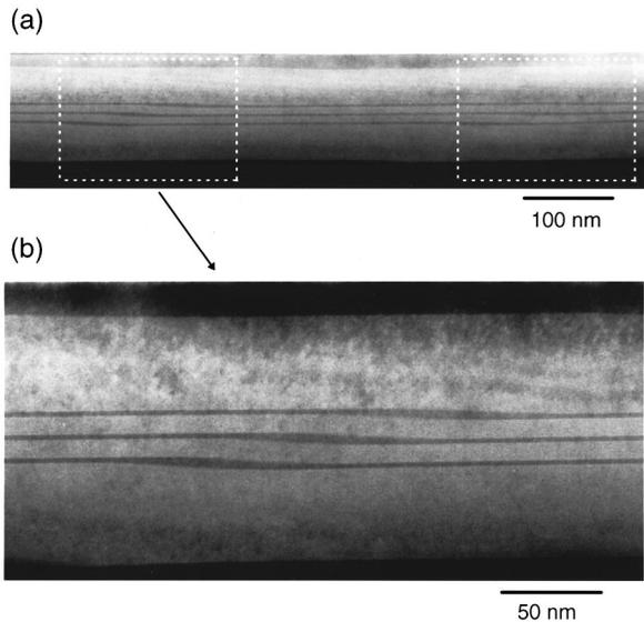
FIG. 1. (a) Cross-sectional TEM image viewed along [01-1] of the 500-nm-pitch array of vertically stacked sidewall quantum wires on patterned GaAs (311)A substrates. In (b) the scale is enlarged.
