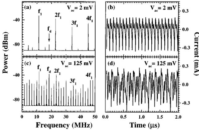
FIG. 1. Current power spectra (left) and real-time current traces (right) for  $V_{ac}=2$  and 125 mV, respectively, recorded at 5 K in a superlattice structure.
