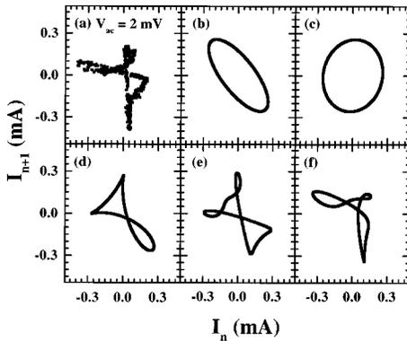
FIG. 2. (a) Experimentally derived Poincaré map for the quasiperiodic oscillations observed at 2 mV. Calculated Poincaré maps for (b) the fundamental frequency  $f_1$  alone, (c) the second harmonic  $f_2$  alone, (d)  $f_1$  and  $f_2$  together, (e)  $f_1$  plus three higher harmonics and no phase shift ( $\phi_1=0$ ), and (f)  $f_1$  plus three higher harmonics and a phase shift of  $\phi_1=0.8\pi$ . The frequency ratio was set to  $f_d/f_1=(1+\sqrt{5})/2$ .
