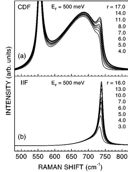
FIG. 3. Theoretical line shapes of Raman spectra for scattering by overdamped plasmon-related excitations according to the CDF (a) and the IIF (b) scattering mechanisms and different cutoff wave vectors  $q_{\text{max}} = r q_{\text{FT}}$ .
