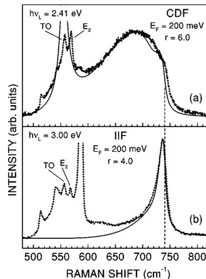
FIG. 1. Polarized Raman spectra (dotted lines) excited at 2.41 eV (a) and at 3.00 eV (b). Theoretical line shapes with a Fermi energy of 200 meV (solid lines) are shown for the CDF (a) and the IIF (b) scattering mechanisms.
