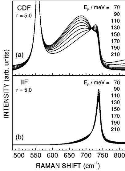
FIG. 2. Theoretical line shapes of Raman spectra for scattering by overdamped plasmon-related excitations according to the CDF (a) and the IIF (b) scattering mechanisms and different Fermi energies  $E_F$ .
