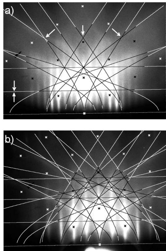
FIG. 2. Kikuchi line fits to diffraction patterns of (a) GaAs (001)  $\beta(2 \times 4)$  and (b) AlAs (001)  $c(4 \times 4)$  reconstructed surfaces. Arrows indicate the most reliable points for fitting.
