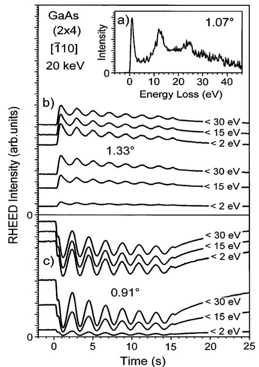
FIG. 4. RHEED intensity oscillations for GaAs (001) growth recorded on the specular spot along  $[210]$  with different inelastic components included. The inset (a) shows a typical energy loss spectrum.
