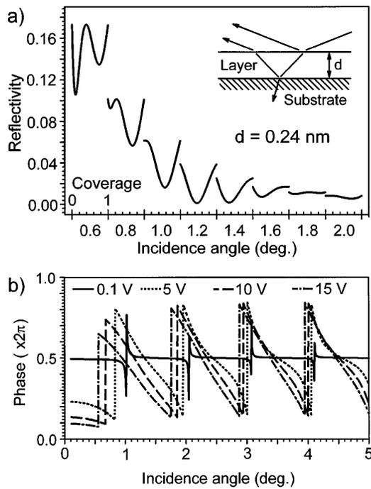
FIG. 1. Layer interference model. The reflectance change during the deposition of one layer is shown in (a) for different incidence angles together with the geometry used for the calculations. Two amplitude minima at  $\approx 0.7^\circ$  and  $\approx 1.8^\circ$  are shown. Phase dispersion plots (position of the oscillation minimum as a function of incidence angle) for different potential values are given in (b).
