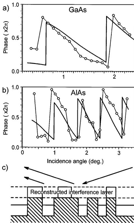
FIG. 3. Comparison of experimental data recorded in the one-beam condition with layer thickness fits obtained from the layer interference model. In (a), a value of  $d = 0.24$  nm is obtained; the result in (b) is  $d = 0.38$  nm. The different thicknesses obtained for materials with practically identical bulk lattice constants leads to the model shown in (c), where the interference takes place in the surface reconstruction on top of the growing layer.
