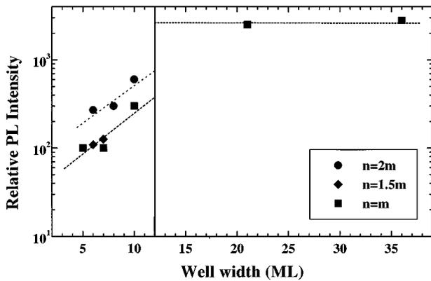
FIG. 2. Integrated PL intensity vs well width for the symmetric (squares), asymmetric with  $n=1.5m$  (diamonds), and asymmetric with  $n=2m$  SLs (dots). The vertical solid line indicates the well width for the  $\Gamma$ - $X$  crossover in symmetric SLs.
