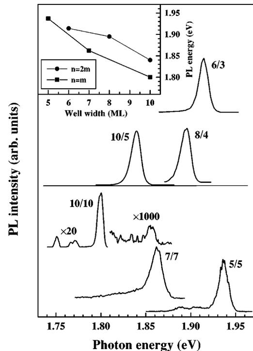
FIG. 1. PL spectra of the symmetrical (lower part) and asymmetrical (upper part) SLs recorded at 4.2 K. The spectra of the different samples were normalized to their respective maximum intensity. The inset shows the energetic positions of the maximum PL vs the well width.
