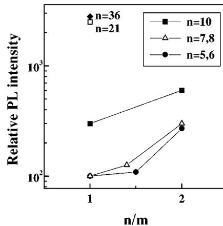
FIG. 3. Integrated PL intensity vs ratio of well-to-barrier width in ML for all samples shown in Fig. 2 as indicated.
