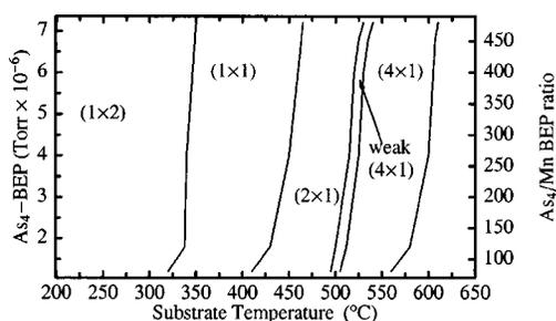
FIG. 2. Surface phase diagram for MnAs( $\bar{1}100$ ) growth from Mn and  $As_4$  molecular beams. MnAs growth rate:  $10 \text{ nm h}^{-1}$ .
