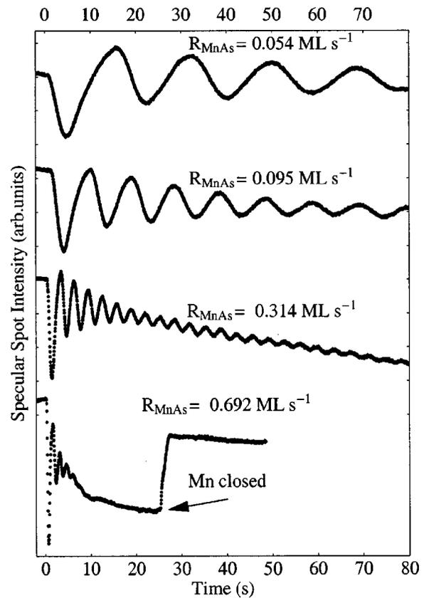
FIG. 3. RHEED intensity oscillations of the specular spot measured in the MnAs  $[11\bar{2}0]$  azimuth as a function of growth rate  $R_{MnAs}$ . The surface was grown at a substrate temperature of  $265^\circ\text{C}$  after a short annealing at  $300^\circ\text{C}$ . The Mn flux was applied at  $t = 0$ .
