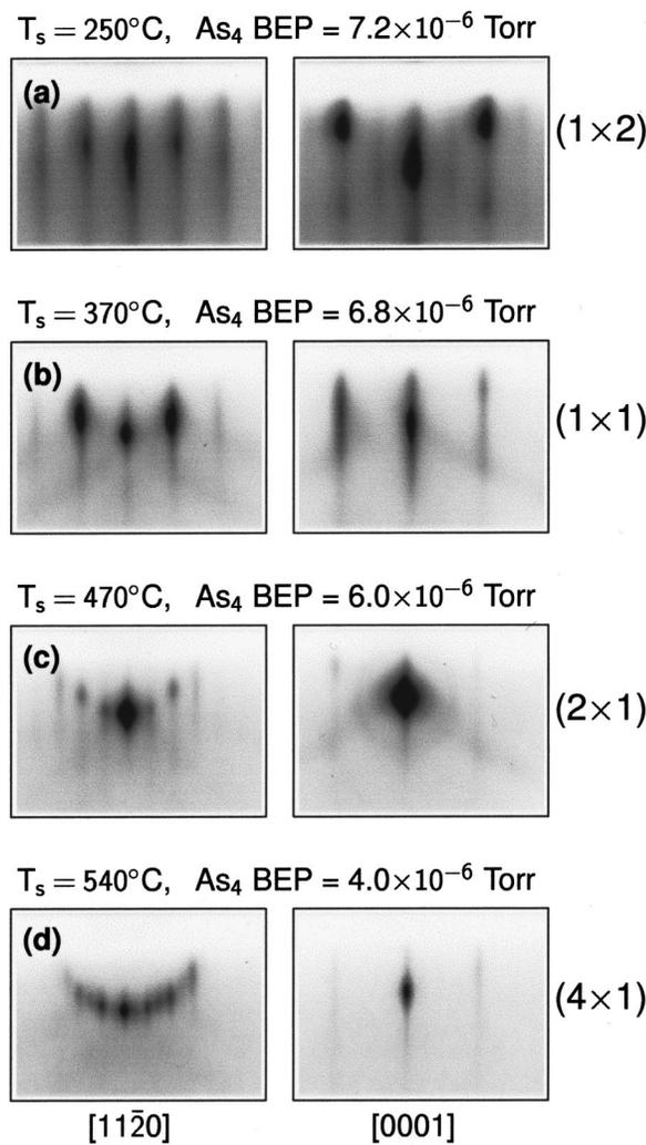
FIG. 1. Characteristic RHEED patterns of MnAs( $\bar{1}100$ ) along the  $[11\bar{2}0]$  azimuth (left panels) and  $[0001]$  azimuth (right panels) recorded during growth at different substrate temperatures and  $As_4$  BEP values. MnAs growth rate:  $10 \text{ nm h}^{-1}$ .
