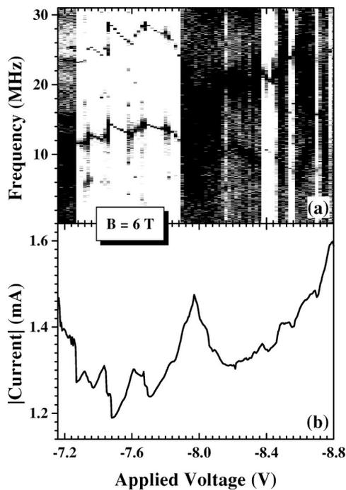
FIG. 3. Power spectra of the self-sustained oscillations (a) vs applied voltage and time-averaged  $I$ - $V$  characteristic (b) recorded at  $B = 6$  T.
