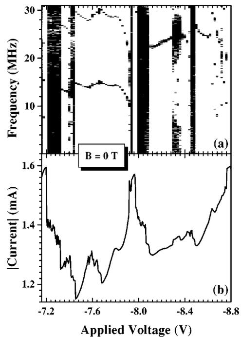
FIG. 2. Power spectra of the self-sustained oscillations (a) vs applied voltage and time-averaged  $I$ - $V$  characteristic (b) recorded at  $B=0$  T.
