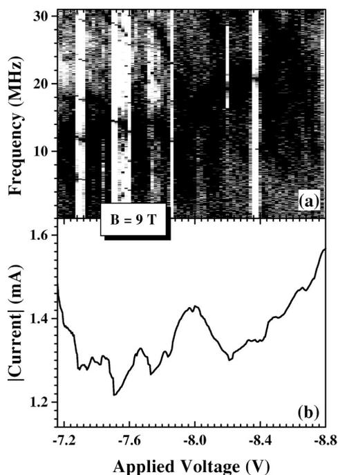
FIG. 4. Power spectra of the self-sustained oscillations (a) vs applied voltage and time-averaged  $I$ - $V$  characteristic (b) recorded at  $B = 9$  T.
