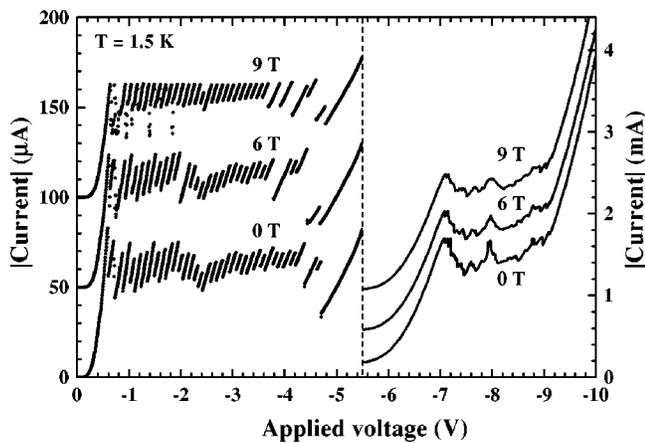
FIG. 1. Time-averaged  $I$ - $V$  characteristics recorded at 1.5 K for  $B=0$ , 6, and 9 T. The traces for voltages between 0 and  $-5.5$  V ( $-5.5$  and  $-10$  V) recorded at 6 and 9 T have been shifted upward by 50 and 100  $\mu$ A (0.5 and 1.0 mA), respectively.
