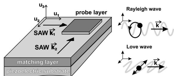
FIG. 3. Sketch of the investigated material system: a matching layer is deposited on top of the piezoelectric substrate and a probe layer is placed in some distance from the IDTs. The wave displacement components ( $u_1, u_2, u_3$ ) for the two wave types are shown on the rhs.;  $u_1$  is along the propagation direction. The Rayleigh-type wave is predominantly polarized in the  $u_1 - u_3$  plane, whereas the Love wave only has an in-plane ( $u_2$ ) oscillation component.
