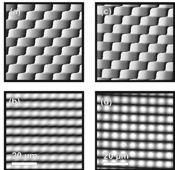
FIG. 2. SAW phase (a),(c) and amplitude (b),(d) patterns of a Rayleigh-type wave field obtained by a SAFM mixing experiment. (a) and (b) show the simulated data and (c) and (d) the experimental data, respectively. Two rf generators were used to power three of the four IDTs, while the fourth is acting as a wave reflector to establish a partly standing wavefield.
