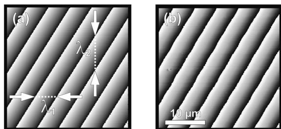
FIG. 4. (a) Simulated and (b) measured SAFM phase image. The mixing experiment was carried out using a Rayleigh-type wave (propagating from right to left) and a Love wave (propagating from top to bottom).
