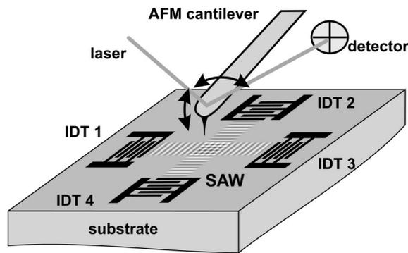
FIG. 1. Sketch of the SAFM experimental setup: detuned rf surface acoustic waves are launched by IDTs on a piezoelectric substrate towards the measurement region, where a down conversion at the tip-sample contact takes place. The resulting vertical and lateral 1f cantilever oscillations are optically detected and analyzed by a lock-in amplifier. Phase and amplitude are recorded along with the topography scan.
