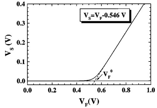
FIG. 4. Surface photovoltage  $V_S$  as a function of surface Fermi voltage  $V_F$  calculated using Eq. (1) with the parameters  $A^*=2.4 \times 10^5 \text{ A(m K)}^{-2}$ ,  $B=4.63 \times 10^{-5} \text{ K}^{-3/2}$ ,  $J_{PC}=11.4 \text{ A m}^{-2}$ ,  $T=300 \text{ K}$ , and  $\eta=1$ .
