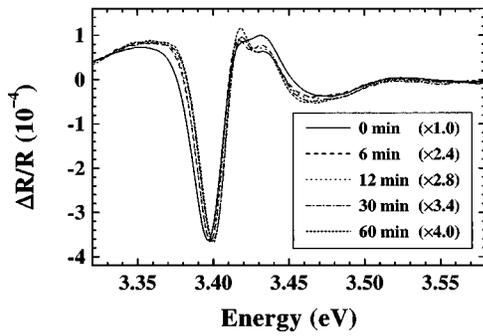
FIG. 1. Photorefectance spectra of the GaN film measured at different times as indicated after starting the evacuation of the cryostat at 300 K. For a better comparison, the amplitude of all spectra has been normalized to the spectrum taken without evacuation (0 min).
