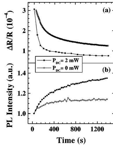
FIG. 2. (a) PR amplitude and (b) integrated photoluminescence intensity as a function of evacuation time of the cryostat without and with additional unmodulated UV illumination for the same sample as in Fig. 1 measured at 300 K.
