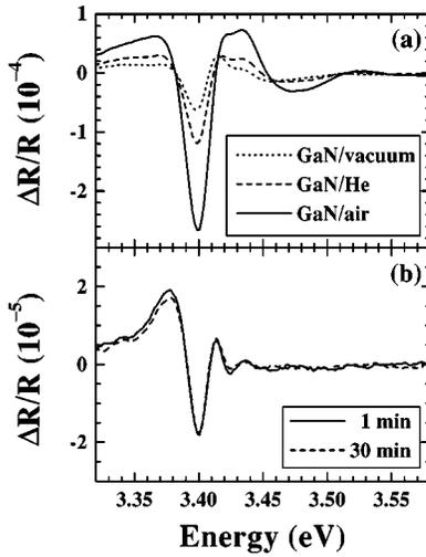
FIG. 3. PR spectra for different ambient media on the same sample as in Fig. 1 as indicated (a) and for the sample with a 7 nm Ti layer measured at different evacuation times as indicated with additional UV illumination (b) at 300 K.
