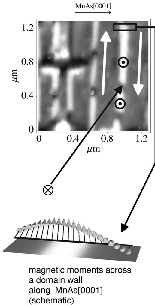
FIG. 6. MFM measurement of a domain boundary. The orientation of two neighbored domains is indicated by white arrows. The direction of the magnetic moments in the domain wall is shown by in-plane ( $\otimes$ ) and out-of-plane ( $\odot$ ) pointers, respectively. The pointers are schematically emphasized on the right hand side, representing a cross section of the wall.
