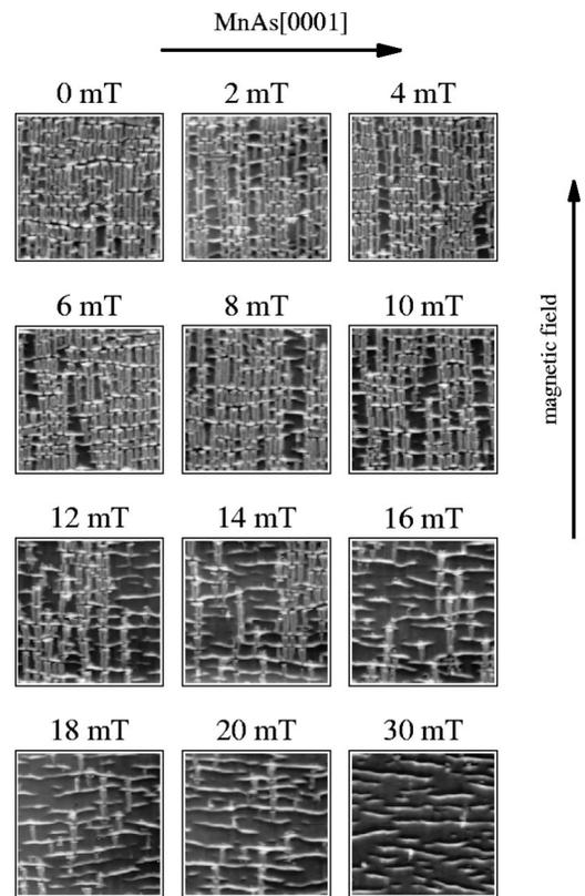
FIG. 7. MFM images of the  $\text{MnAs}(\bar{1}100)$  surface taken over a scan area of  $10 \mu\text{m} \times 10 \mu\text{m}$ . The images have been obtained after applying a magnetic field outside of the MFM instrument with different field strengths parallel to  $\text{MnAs}[11\bar{2}0]$ . The field strength used to magnetize the sample is indicated in every image.
