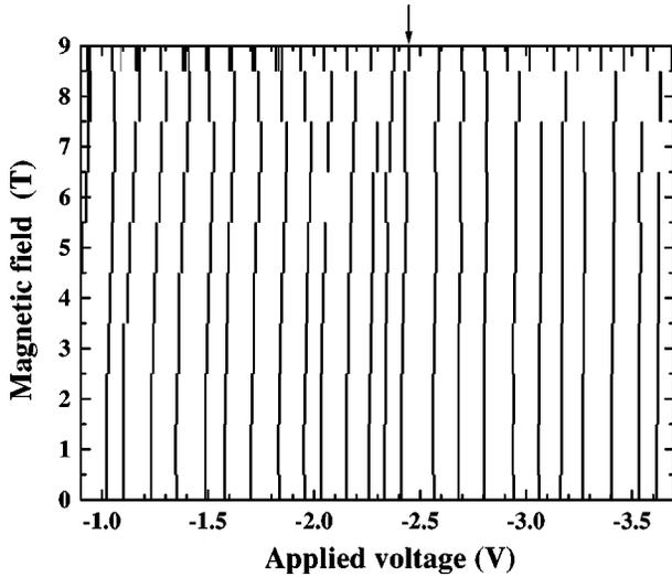
FIG. 2. Grey scale plot of the differential conductance  $dI/dV$  versus applied voltage and magnetic field.  $dI/dV$  has been obtained numerically from the I-V characteristics recorded for the same condition as in Fig. 1. The darker areas indicate the regions of negative differential conductance.
