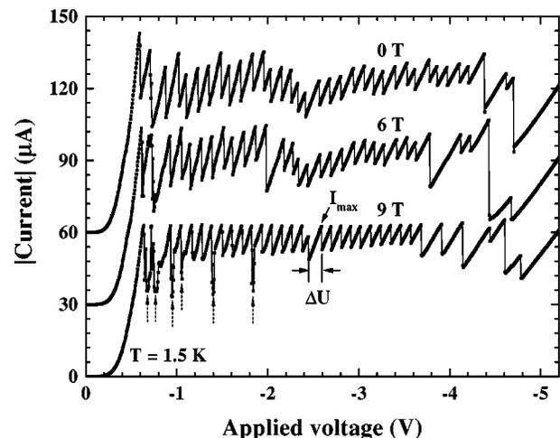
FIG. 1. Time-averaged I-V characteristics at 1.5 K for several magnetic fields as indicated. The solid lines are a guide to the eye. For clarity, the traces at 6 and 0 T have been shifted upwards by 30 and 60  $\mu\text{A}$ , respectively.
