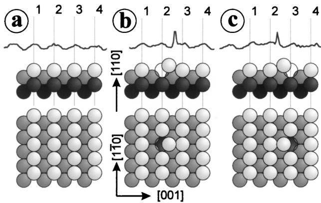
FIG. 3. Line-scan sections from the Ag(110) terraces of Fig. 4d with sphere models in side and top view representation: (a) undisturbed terrace (section of scan 317); (b), (c) atomic jumps from fcc to hcp sites (sections of scan 494 and 400, respectively).
