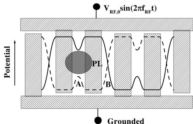
FIG. 1. Structure of the interdigitated metal gates and potential distributions in the quantum well under positive (solid line) and negative (dashed line) biases.
