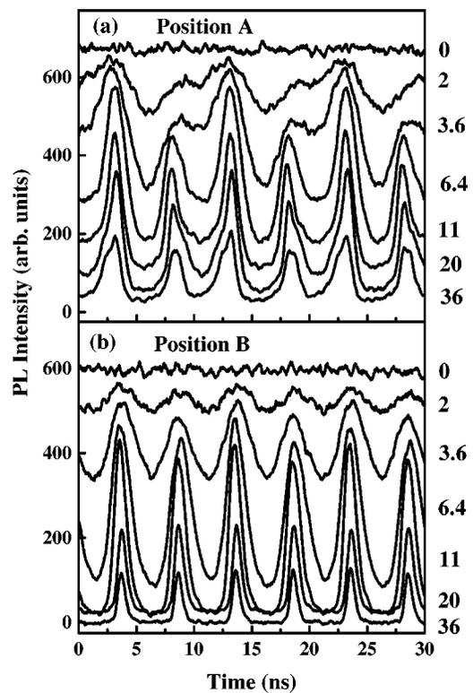
FIG. 4. PL traces measured under a rf excitation of 100 MHz for different rf voltages at (a) position A and (b) position B.
