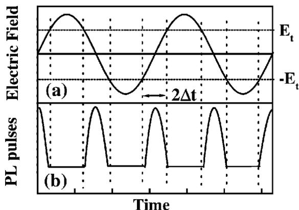
FIG. 3. Schematic time dependence of the electric field (a) and of the PL intensity (b).
