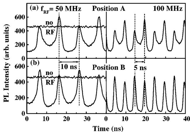
FIG. 2. Pulsed PL traces measured for  $f_{\text{rf}}=50$  MHz (left) and  $f_{\text{rf}}=100$  MHz (right) and for a rf voltage of 11 mV at (a) position A and (b) position B.
