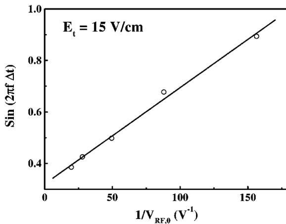
FIG. 5.  $\sin(2\pi f \Delta t)$  vs  $1/V_{rf,0}$  for position B. The data have been obtained from Fig. 4(b). The solid line is a linear fit to the data points.
