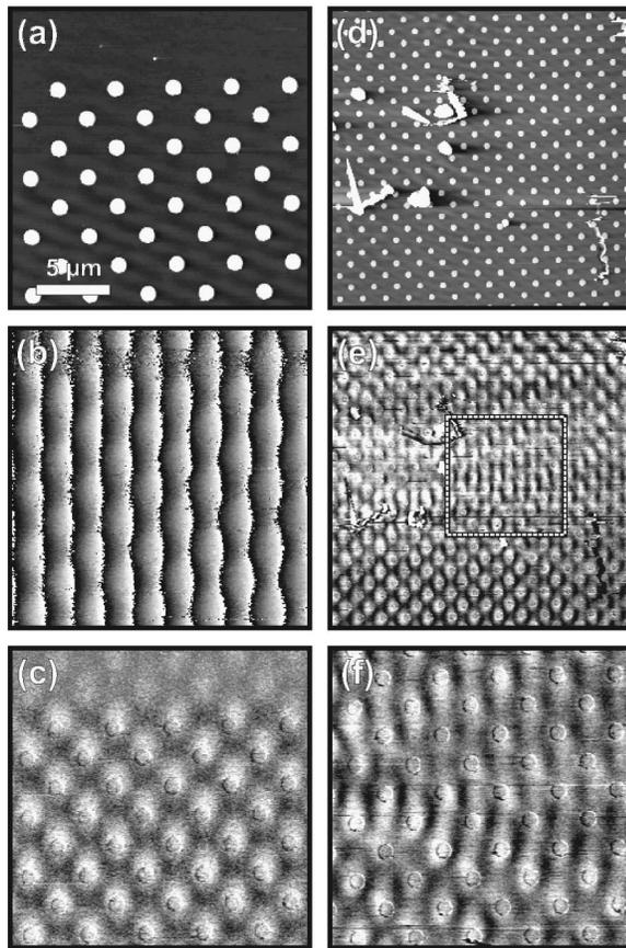
FIG. 3. Topographies (a), (d), phase (b), and amplitude (c), (e), (f) SAFM scans of a 2D scattering dot array (Au,  $d=1\ \mu\text{m}$ ; fcc,  $\Delta x=4\ \mu\text{m}$ ;  $\lambda_{\text{SAW}}=4.0\ \mu\text{m}$ ). Images (a)–(c) show the results for the periodic array, and (d)–(f) the results for the locally damped array.
