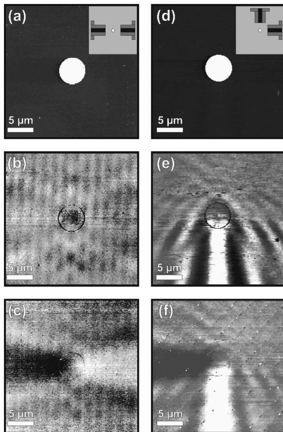
FIG. 2. SAFM topography (a), (d), amplitude (b), (e), and phase deviation (c), (f) of a scattering dot (Au, diameter  $5 \mu\text{m}$ ) on (001) GaAs for  $0^\circ$  (a)–(c) and  $90^\circ$  (d)–(f) sampling geometries. The SAWs were launched along  $[100]$  directions ( $+5 \text{ dBm}$ , from the bottom or left and  $-5 \text{ dBm}$ , from the right) with  $\lambda_{\text{SAW}} = 3.3 \mu\text{m}$ .
