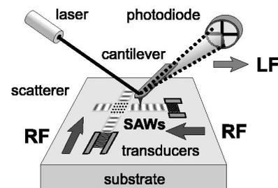
FIG. 1. Schematic representation of the SAFM.
