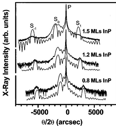
FIG. 1. X-ray rocking curves (004) of InP/GaP superlattices with different InP coverage along with respective simulations (solid lines). The best fits are obtained using  $d_{\text{GaP}}=42.5 \text{ \AA}$ ,  $d_{\text{InP}}=2.6, 4.0, \text{ and } 5.3 \text{ \AA}$  for the lower, middle, and top curves, respectively. With decreasing InP coverage, the zeroth order superlattice satellite ( $S_0$ ) shifts from  $-2000$  to  $-1000$  arcsec towards the GaP substrate peak ( $P$ ).
