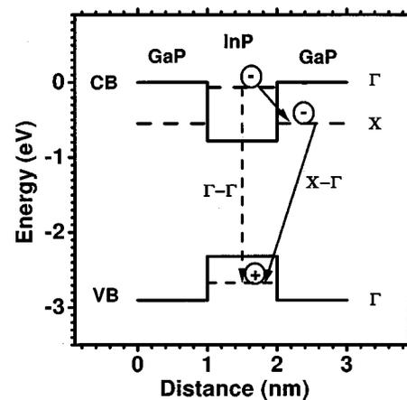
FIG. 3. Valence and conduction band alignment scheme of the InP QW embedded in a GaP matrix. The arrows indicate the two possibilities of electron-hole recombination.
