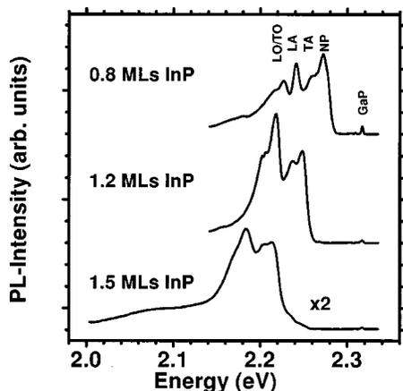
FIG. 2. Photoluminescence spectra of samples with different InP coverage measured at 5 K.
