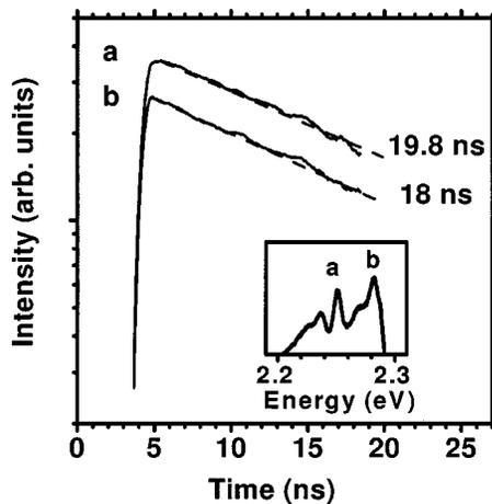
FIG. 4. PL transients from the sample with 0.8 MLs InP coverage. The transients were detected at 2.24 (a) and 2.27 (b) eV and 5 K. The dashed lines show the fit with the corresponding time constant. The inset shows the PL spectrum with the positions of the detection energies marked by a and b.
