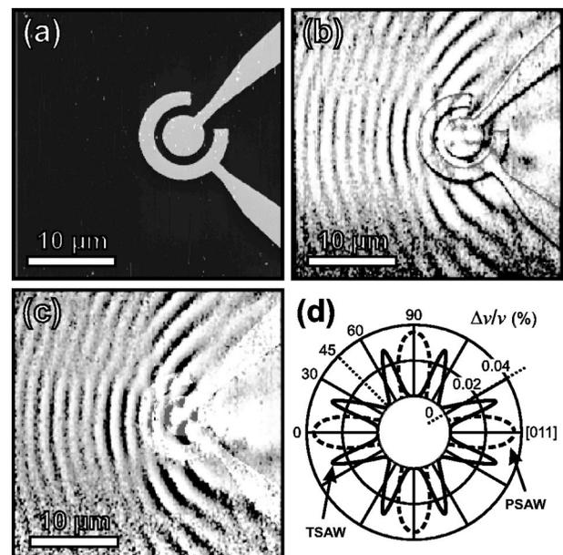
FIG. 3. Circular single source [Al electrodes, inner diameter:  $4 \mu\text{m}$ , gap width:  $1 \mu\text{m}$ , (001) GaAs]: (a) topography, (b) amplitude, and (c) phase image. The plane sample wave was launched from the left at 890 MHz ( $\lambda = 3.2 \mu\text{m}$ ). The amplitude (b) and phase (c) images show the excited wave field with the preferred excitation directions. (d) Polar plot of the electro-mechanical coupling coefficient for the true SAW (TSAW) and the pseudo SAW (PSAW).
