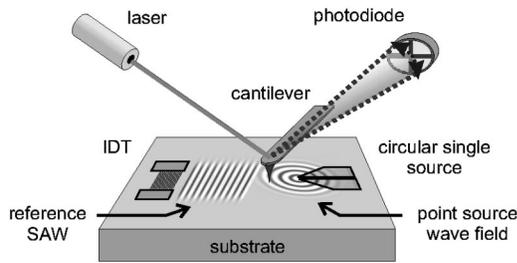
FIG. 1. Sketch of the SAFM experimental setup. The reference plane wave is launched towards the tip for sampling the complex radiation pattern of the single circular source.
