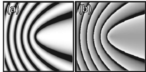
FIG. 2. Simulation of the SAFM amplitude (a) and phase (b) signal for the mixing of a plane wave with the wave field of an ideal circular source (without taking the substrate anisotropy or the electromechanical coupling strength into account).
