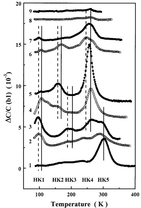
FIG. 3. Deep-level spectra (Fourier coefficient  $b_1$ , 100 ms pulse width, 1 s period) for as-grown GaAs/Ga(As,N)/GaAs structure No. 1. Spectra 1–9, which correspond to increasing quiescent biases, are vertically shifted for clarity. The pulse height was 0.5 V. For hole traps HK1–HK5 in Ga(As,N) and GaAs, the temperature positions of the DLTFs peaks are marked by dashed and solid lines, respectively.
