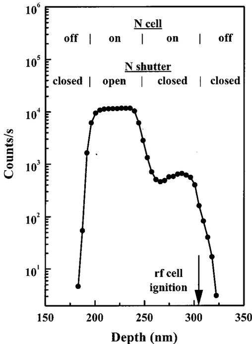
FIG. 1. Typical depth profile of nitrogen measured by SIMS for as-grown sample No. 1. The rf plasma ignition point is indicated by the arrow. The operation of the N cell and the position of the N shutter are sketched for the different regions.
