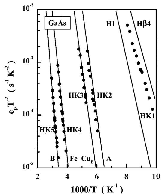
FIG. 8. Arrhenius plots for hole traps HK1, HK2, HK3, HK4, and HK5 in the GaAs layers of GaAs/Ga(As,N)/GaAs heterostructures (dots) compared with published data (lines) for the irradiation-induced hole traps, H $\beta$ 4 (Ref. 22) and H1 (Ref. 23), the two levels A and B typical of LPE-grown GaAs (Ref. 24), the Cu<sub>B</sub> level (Ref. 25), and the trap due to Fe in GaAs (Refs. 26).
