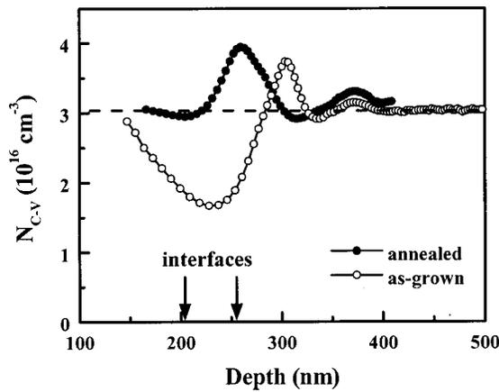
FIG. 2. Typical depth profiles of the apparent hole concentration  $N_{C-V}$  for as-grown and annealed GaAs/Ga(As,N)/GaAs structures. The plots were measured at 300 K and 1 MHz for the GaAs/Ga(As,N)/GaAs structure with undoped Ga(As,N) (sample No. 1). The dashed line indicates constant doping level of  $3 \times 10^{16} \text{ cm}^{-3}$  in the entire heterostructure. The positions of the two heterointerfaces are marked by arrows.
