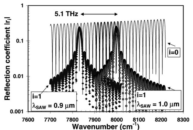
FIG. 6. Absolute value of the complex reflection coefficient of the structure in Fig. 2 for the unshifted ( $|r_0|$ , solid line) and for the up-shifted ( $|r_1|$ , symbols) beams under modulation by a SAW with wavelengths of  $\lambda_{\text{SAW}} = 1.0 \mu\text{m}$  (diamonds) and  $\lambda_{\text{SAW}} = 0.9 \mu\text{m}$  (circles). The oscillations in the spectra arise from Fabry–Perot interference fringes in the total length  $l_W = 100 \mu\text{m}$  of the structured waveguide.
