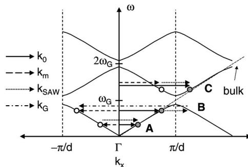
FIG. 3. Light dispersion in a periodically structured material displaying normal (A) and umklapp scattering processes (B and C). The arrows display the wave vectors of the incident light ( $k_0$ , solid arrow), of the diffracted light ( $k_m$ , dashed arrow), of the SAW ( $k_{\text{SAW}}$ , dotted arrow), and the grating wave vector  $k_G = 2\pi/d$  (dash-dotted arrow).
