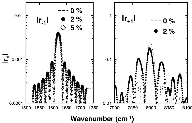
FIG. 7. Wave number dependence of the reflection ( $|r_m|$ ) coefficients of the first (left panel) and second (right panel) Bragg reflection peaks in Fig. 5 including the effect of random fluctuation of the lateral sizes  $d_1$  and  $d_2$  in Fig. 2. The disorder is quantified in terms of the standard deviation in the lateral sizes of 0% (dashed line), 2% (dots), and 5% (diamonds).
