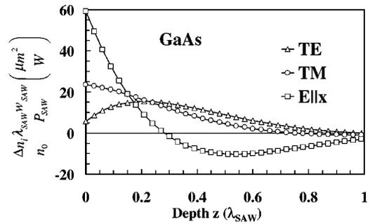
FIG. 4. Depth dependence of the refractive index modulation  $\Delta n_i/n_0$  by a SAW in GaAs for TE (electric field  $E$  parallel to  $y = [1\bar{1}0]$ ) corresponding to  $i=2$ ) and TM ( $E||z=[001]$ ,  $i=3$ ) polarizations, and for  $E||x=[110]$  ( $i=1$ ).
