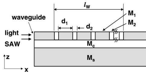
FIG. 2. Structure of a Bragg reflection cell using a periodically structured medium composed of materials  $M_1$  and  $M_2$ .  $M_c$  and  $M_s$  denote the cladding layer and substrate, respectively.  $l_w$  denotes the length of the modulated region of the waveguide.
