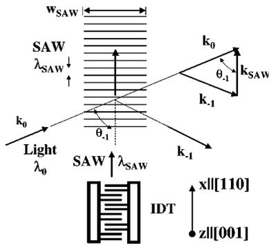
FIG. 1. Bragg diffraction of a light beam on a surface acoustic wave generated by an interdigital transducer (IDT).
