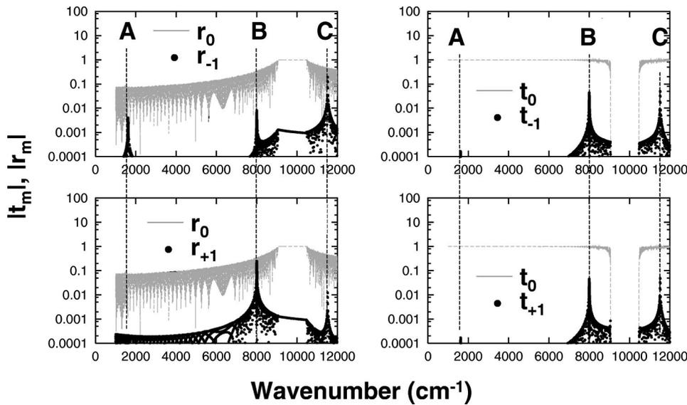
FIG. 5. Wave number dependence of the reflection ( $|r_m|$ , left panels) and transmission ( $|t_m|$ , right panels) coefficients for collinear Bragg reflection on a SAW. The apparent scattering in the data points arise from Fabry–Perot interference fringes in the length  $l_W$  of the modulated waveguide (see Fig. 2).
