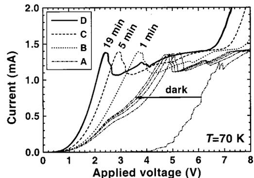
FIG. 4.  $I-V$  characteristics of sample A for voltage sweeps from 0 to 8 V for different illumination conditions at 70 K. The set of curves labeled A was recorded successively from right to left without illumination. Curves B and C correspond to voltage sweeps after cumulative illumination for 1 and 5 min, respectively. Curve D was recorded after 19 min of illumination.
