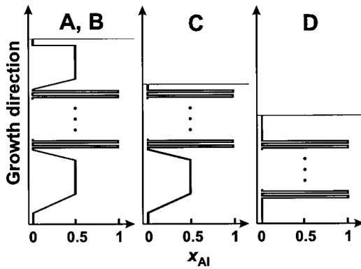
FIG. 1. Sketch of the Al mole fraction  $x_{Al}$  in structures A, B, C, and D.
