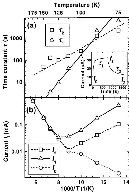
FIG. 5. (a) Rise  $\tau_1$  and decay times  $\tau_2$  as well as (b) saturation currents  $I_0$ ,  $I_1$ , and  $I_2$  vs inverse temperature  $T$  for sample B at a voltage of 2 V and constant LED current. The inset shows a typical current transient.
