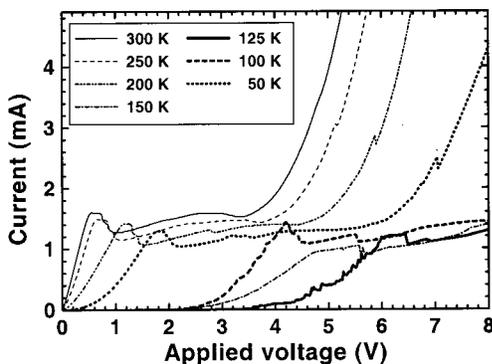
FIG. 2.  $I-V$  characteristics of sample A recorded for the different temperatures indicated. Before the first measurement, 10 V was applied for a few seconds. All sweeps were performed from 0 to 8 V.
