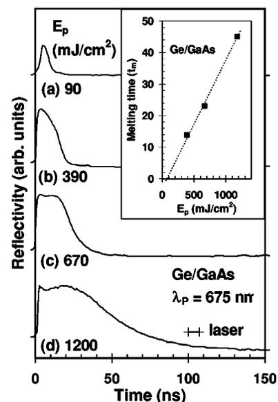
FIG. 2. Time-resolved reflection profiles obtained during the irradiation of Ge films on GaAs with laser pulses with average fluencies  $E_p$  of: (a) 90 mJ/cm<sup>2</sup>, (b) 390 mJ/cm<sup>2</sup>, (c) 670 mJ/cm<sup>2</sup>, and (d) 1200 mJ/cm<sup>2</sup>.
