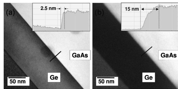
FIG. 6. Dark field TEM micrographs obtained from reflections from the  $\{200\}$  planes perpendicular to the Ge/GaAs interface for fluency regions (a) C and (b) D [cf. Fig. 1(b)]. The insets display intensity profiles of the [200] reflex across the interface recorded along the scan line indicated in the figure.
