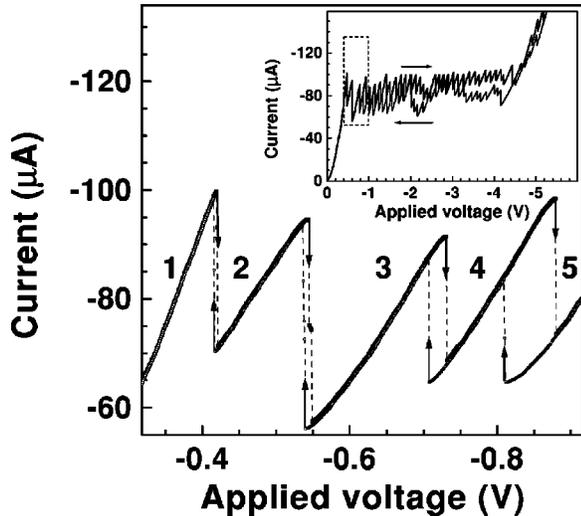
FIG. 1. Time-averaged  $I$ - $V$  characteristics of the first five branches (1, 2, 3, 4, 5) for up sweep and down sweep between 0 and  $-6$  V as indicated by the arrows at 5 K. The full  $I$ - $V$  characteristics for both sweep directions is shown in the inset.
