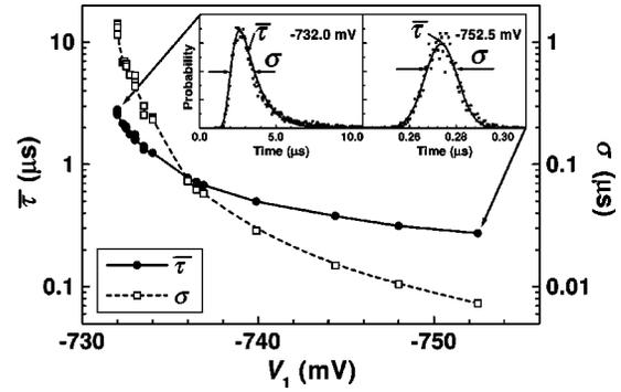
FIG. 3. Average value  $\bar{\tau}$  (dots) and width  $\sigma$  (open squares) of the distribution of the relocation times for switching from  $V_0 = -650$  mV on branch 3 to different final voltages on the branch 4. The insets show two examples of the distribution functions measured at a voltage of  $V_1 = -732$  and  $-752.5$  mV.
