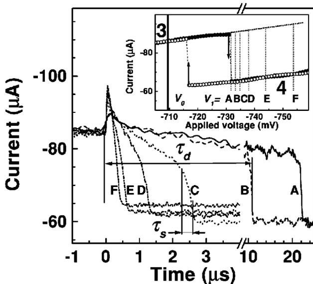
FIG. 2. Typical time traces for switching from  $V_0$  on branch 3 to different voltages (A to F) on branch 4. The switching time  $\tau$  is indicated for case B. The closer the final voltage is to the beginning of the fourth branch, the longer the switching time. The inset displays the time-averaged  $I$ - $V$  characteristics indicating  $V_0$  and the different final voltages  $V_1$  labeled A to F.
