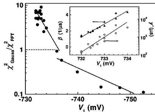
FIG. 5. Ratio of  $\chi_{\text{Gauss}}^2$  to  $\chi_{\text{FPT}}^2$  as a function of final voltage on branch 4. A transition happens at about 735 mV, where the ratio is about unity and the slope of the fitting line changes. The inset displays the dependence of the fitting parameters  $\beta$  (triangles) and  $y'$  (circles) on  $V_1$  for the regime, where the above ratio is larger than one.
