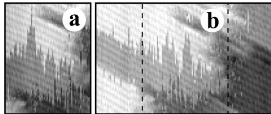
FIG. 2. Subsequent STM images of Au(110): the area displayed in (a) is included in (b) marked by dashed lines; tunneling conditions as in Fig. 1, fast scanning direction vertical.
