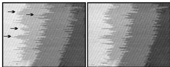
FIG. 1. STM image sections  $[160 \times 125$  data points (dp) of  $256 \times 256]$  of the same Au(110) area taken at  $460 \pm 20$  K obtained from forward (left) and backward scans (right);  $U_T = 688$  mV,  $I_T = 0.2$  nA; scanning speed: 2330 dp/s.
