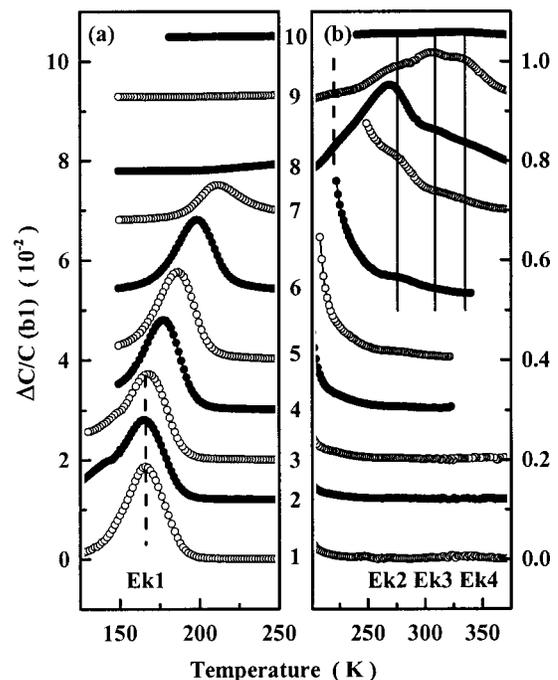
FIG. 1. Typical temperature scans of the DLTFS signal  $\Delta C/C$  for as-grown *n*-type GaAs/Ga(As,N)/GaAs heterostructures (Fourier coefficient  $b_1$ , 1 MHz frequency, 1 s period, 100 ms pulse width). The spectra 1-10 correspond from  $-2$  to  $-6.5 \text{ V}$  to reverse biases increasing in 0.5 V steps with a pulse height of 0.5 V. The peak positions of the traps Ek1-Ek4 are indicated. The  $\Delta C/C$  scale in (b) is expanded by a factor of 10.
