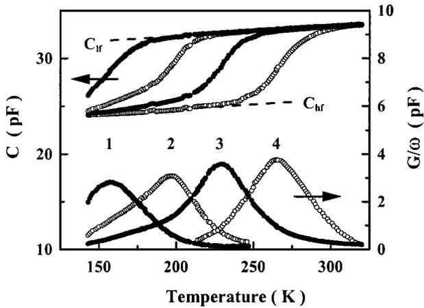
FIG. 2. Typical admittance dispersion for *n*-type GaAs/Ga(As,N)/GaAs structures measured at  $-2$  V and frequencies of (1) 1, (2) 10, (3) 100, and (4) 1000 kHz. The capacitances  $C_{lf}$  and  $C_{hf}$  are indicated.
