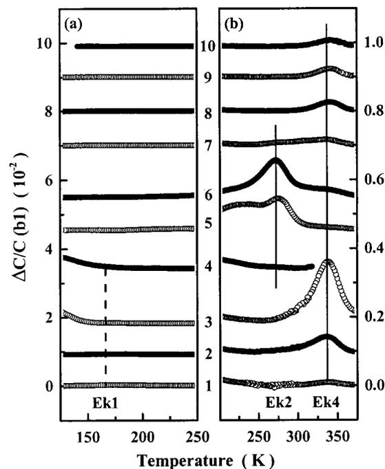
FIG. 4. Deep-level spectra for the same  $n$ -type heterostructure as in Fig. 1, but after postgrowth annealing. Measuring conditions for the spectra 1–10 are identical to those in Fig. 1. Note the same scales as in Fig. 1.
