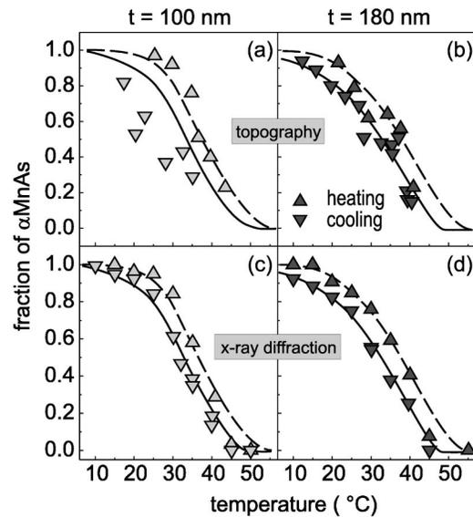
FIG. 2. Fraction of  $\alpha\text{MnAs}$  as a function of sample temperature for a 100-nm-thick (left) and a 180-nm-thick (right) MnAs film as determined from the ridge area fraction of the corrugated MnAs surface (a, b) and by x-ray diffraction (c, d) for heating (triangles up) and cooling (triangles down) of the samples. The solid lines in (c, d) are guides for the eye. For comparison, the same lines are repeated in (a, b).
