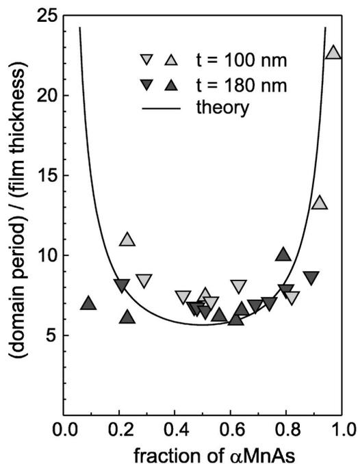
FIG. 4. Surface corrugation period normalized to film thickness as a function of the  $\alpha$ MnAs fraction for both heating (triangles up) and cooling (triangles down) of the samples. The curve is the domain period which minimizes the elastic energy for a given phase fraction.
