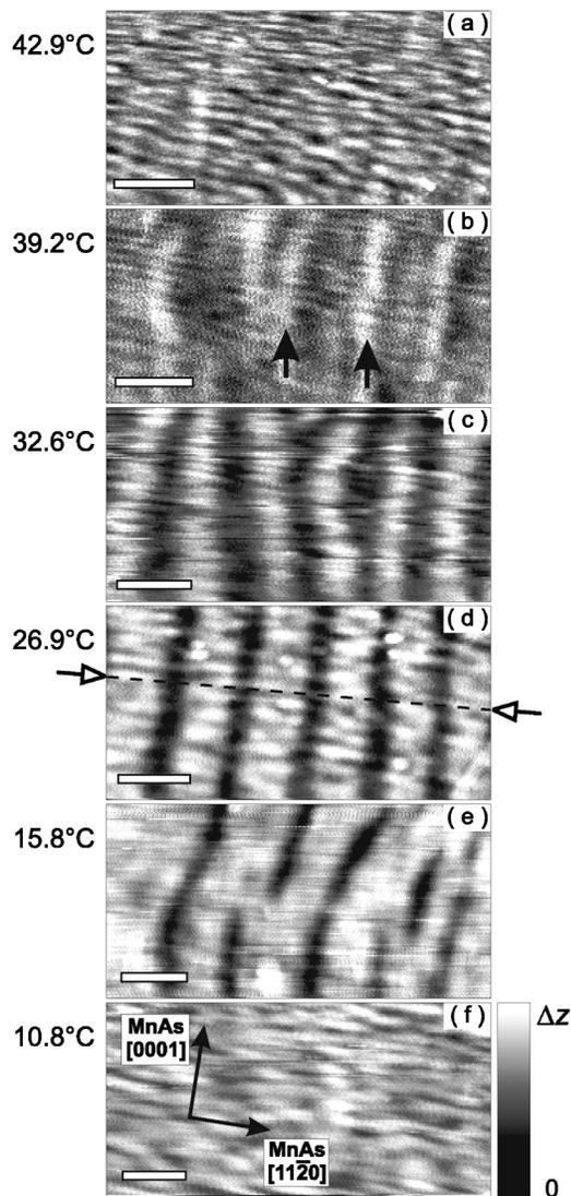
FIG. 1. Surface topography of a 180-nm-thick MnAs film at different sample temperatures. The height ranges  $\Delta z$  are (a) 4.0, (b) 2.8, (c) 3.2, (d) 4.7, (e) 3.4, and (f) 3.8 nm, respectively. In (b) some of the ridges are indicated by arrows. The dashed line in (d) is a line scan taken for Fig. 2. The length of the scale bars is 1  $\mu\text{m}$ .
