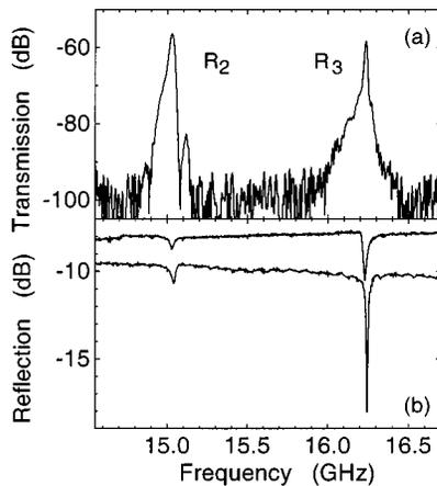
FIG. 1. (a) Transmission and (b) reflection characteristics of delay line #1. The resonances labeled  $R_2$  and  $R_3$  are associated with the second- and third-order Rayleigh modes, respectively.
