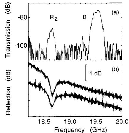
FIG. 2. (a) Transmission and (b) reflection characteristics of delay line #2. The resonance labeled  $R_2$  is associated with the second-order Rayleigh mode. The transmission peak labeled B originates from the scattering of acoustic waves from the sample edge. The curves in (b) are vertically offset for clarity.
