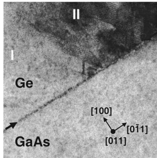
FIG. 5. Details of the lateral interface between the epitaxial (region I) and polycrystalline areas (region II) of LIC Ge/GaAs gratings. The defects in region II consist of twins and stacking faults oriented along  $\{111\}$  planes.
