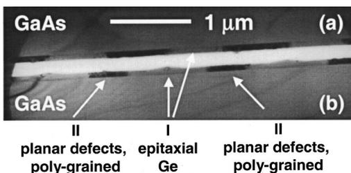
FIG. 4. TEM micrograph of LIC Ge/GaAs gratings produced using (a) low and (b) moderate laser fluencies. For the TEM measurements, the Ge/GaAs structures were glued against each other using an epoxy (white area).
