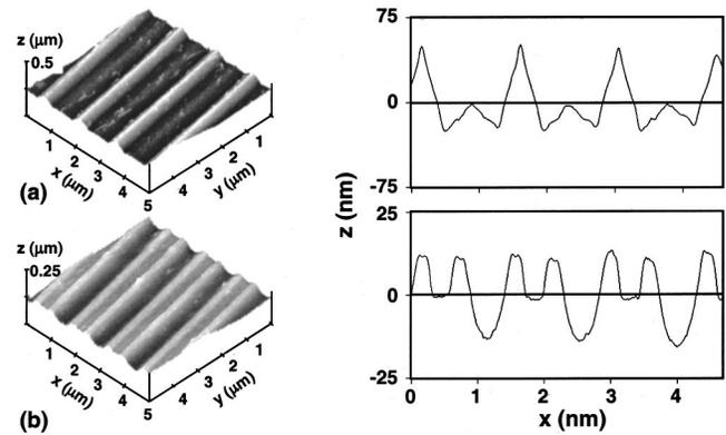
FIG. 2. Atomic force micrographs (left panel) and surface profiles (right panel) of line gratings corresponding to the SEM micrographs in (a) Fig. 1(c) and (b) Fig. 1(d), respectively.
