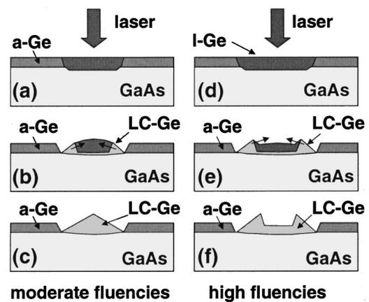
FIG. 6. Schematic sequence of events during the LIC process for moderate (left panel) and high laser fluencies (right panel) showing the selective laser melting [(a) and (d)], the lateral growth [(b)–(e)], and the final structure of the samples [(c)–(f)].
