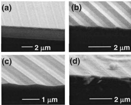
FIG. 1. Scanning electron micrographs of LIC Ge lines on GaAs produced using (a) low, (b) and (c) moderate, and (d) high laser fluencies. The micrographs were recorded at different positions on the spot with a diameter of  $\sim 4$  mm created on the sample surface by LIC using an average laser fluency of  $70 \text{ mJ/cm}^2$ .
