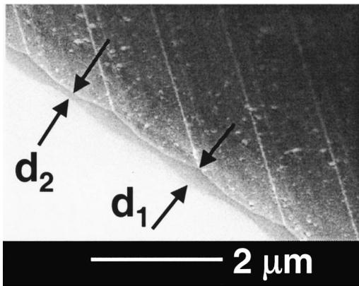
FIG. 3. Cross-sectional SEM micrograph of a grating formed using a moderate laser fluency [corresponding to Fig. 1(b)]. The micrograph was recorded under an observation angle of  $30^\circ$  with respect to the normal to the cleaved edge.
