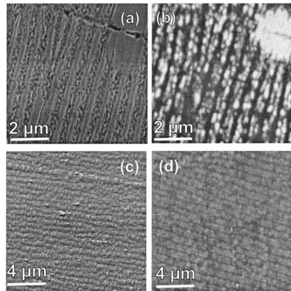
FIG. 5. Room-temperature plane-view SEM micrograph of sample A (a) and a CL map obtained from the same region at 5 K, detected at the wavelength of the  $X$  line (b); room-temperature plane-view SEM micrograph of sample B (c) and a CL map at 5 K, detected at the wavelength of the DAP line (d).
