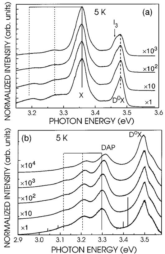
FIG. 8. Excitation density-dependent PL spectra of sample A (a) and sample B (b) at a fixed temperature of 5 K. The unit generation rate in (a) and (b) is  $9 \times 10^{15}$  and  $8.35 \times 10^{15} \text{ cm}^{-2} \text{ s}^{-1}$ , respectively. The equidistant phonon replicas are indicated by vertical lines.
