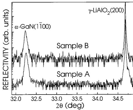
FIG. 3.  $\omega$ - $2\theta$  triple crystal scans across the  $(1\bar{1}00)$  GaN reflection of samples A and B.
