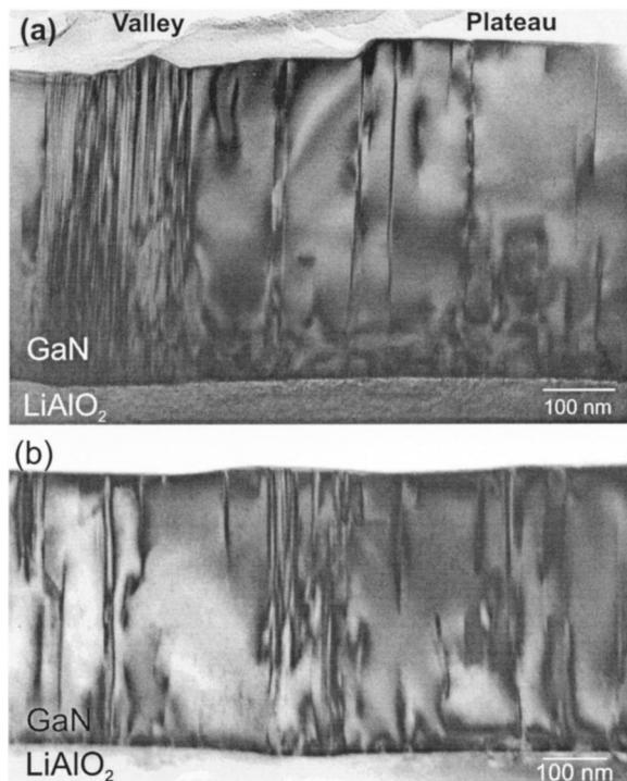
FIG. 7. Cross-sectional  $g = 1\bar{1}00$  two-beam bright-field TEM micrographs near the  $[11\bar{2}0]$  zone axis of sample A (a) and sample B (b). The defects running through the layers are identified as basal plane stacking faults.
