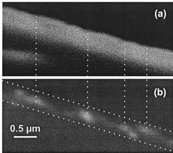
FIG. 6. Cross-sectional SEM micrograph recorded at 5 K (a) and the corresponding CL map of the same region, detected at the wavelength of the X line (b) of sample A.
