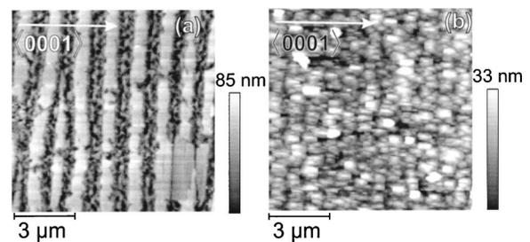
FIG. 2.  $10 \times 10 \mu\text{m}^2$  AFM micrographs of the surfaces of two  $M$ -plane GaN films: sample A (a) and sample B (b).
