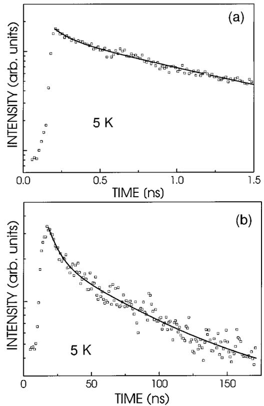
FIG. 11. PL transients of the SF emission from sample A (a) and the DAP transition from sample B (b) recorded at 5 K.
