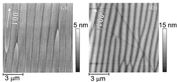
FIG. 1.  $10 \times 10 \mu\text{m}^2$  AFM micrographs of the surface of a typical as-received LAO(100) substrate (a) and after heating in vacuum to  $750^\circ\text{C}$  (b).
