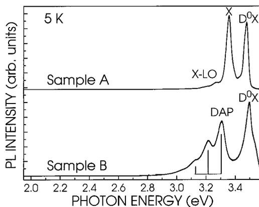
FIG. 4. Photoluminescence spectra of samples A and B recorded at 5 K. The equidistant phonon replicas are indicated by vertical lines.
