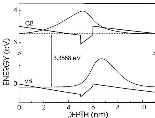
FIG. 10. Band profile, energy states, and electron-hole wave functions of a type II SF in a wurtzite GaN matrix.
