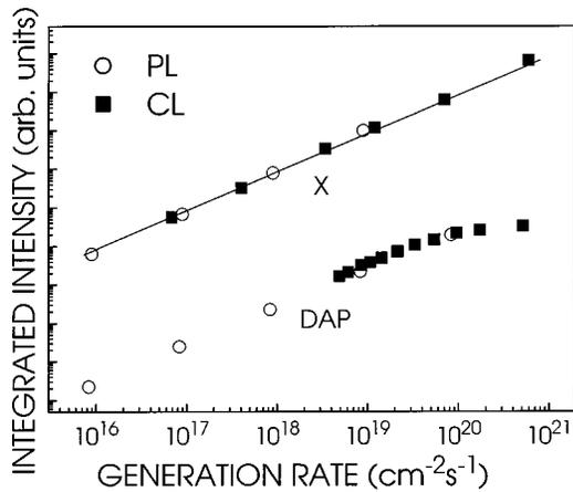
FIG. 9. Integrated PL and CL intensity of the low energy bands in sample A (X) and B (DAP) vs the generation rate. The solid line is a linear fit with a slope of 1.0. The experimental data for PL and CL are vertically offset for clarity.
