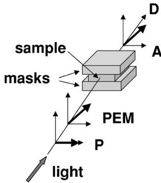
FIG. 3. Experimental setup for TDS measurements in the waveguide geometry:  $P$ , polarizer;  $PEM$ , photoelastic modulator;  $A$ , analyzer; and  $D$ , detector. The sample is sandwiched between two masks of opaque material, which prevents stray light from reaching the detector.
