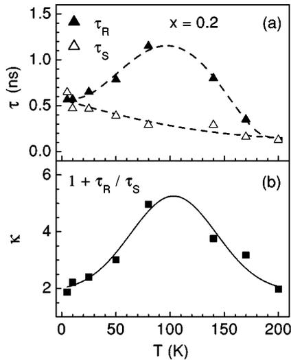
FIG. 3. (a) Measured carrier lifetime  $\tau_R$  (full triangles) as well as spin-relaxation time  $\tau_S$  (open triangles) and (b) the correction factor  $\kappa = 1 + \tau_R/\tau_S$  (full squares) as a function of sample temperature for an (In,Ga)As QW structure with an In content of 0.2. The solid and dashed lines are guides to the eye.
