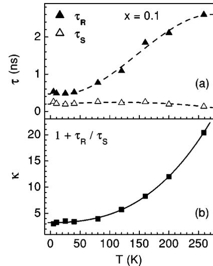
FIG. 4. (a) Measured carrier lifetime  $\tau_R$  (full triangles) as well as spin-relaxation time  $\tau_S$  (open triangles) and (b) the correction factor  $\kappa = 1 + \tau_R/\tau_S$  (full squares) as a function of sample temperature for an (In,Ga)As QW structure with an In content of 0.1. The solid and dashed lines are guides to the eye.
