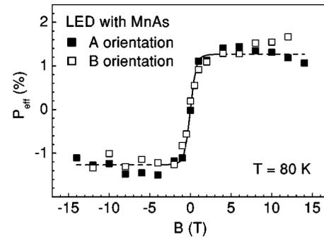
FIG. 2. Effective polarization degree  $P_{eff}$  as a function of external magnetic field measured at 80 K from LEDs with MnAs injection layers of A orientation (full squares) and B orientation (open squares). The contribution due to the Zeeman splitting in the LED layers has been subtracted. The magnetization curve of a thin MnAs layer is shown for comparison in arbitrary units (solid line; dashed line is the continuation as a guide to the eye).
