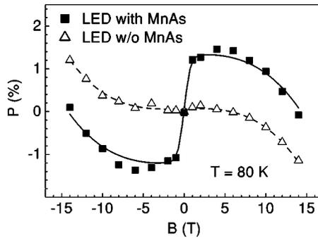
FIG. 1. Circular polarization degree  $P$  as a function of external magnetic field measured at 80 K from LEDs with (full squares) and without (open triangles) a MnAs injection layer. The solid and dashed lines are guides to the eye.
