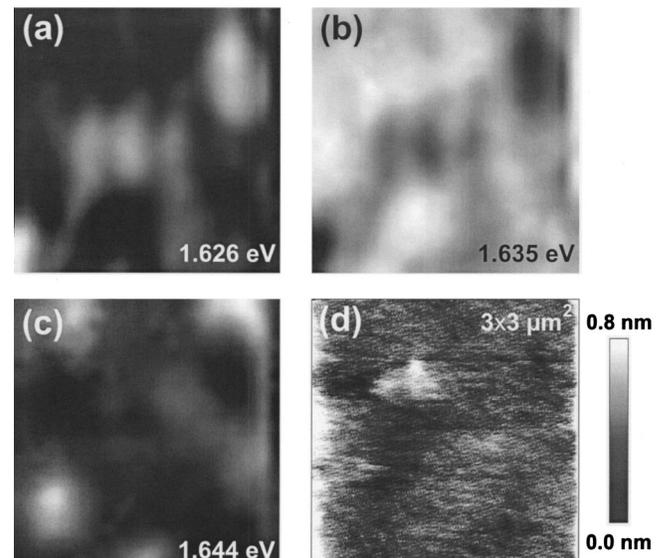
FIG. 5. NFO images of the PL peaks (a) A, (b) B, as well as (c) C in Fig. 4 of the GaAs SQW, and (d) the corresponding shear-force topography image recorded at  $T=13$  K.
