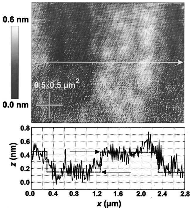
FIG. 3. Shear-force topography image of the sample surface of the GaAs SQW recorded at  $T=13$  K. The line scan across the image (white arrow) shown on the bottom reveals a mean step height of 0.3 nm between two adjacent islands.
