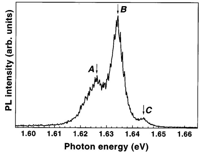
FIG. 4. PL spectrum of the GaAs SQW measured in near-field optical illumination/collection mode at  $T=13$  K. Due to ML thickness fluctuations at both QW interfaces, the PL line is split into three bands at 1.626 (A), 1.635 (B), and 1.644 eV (C).
