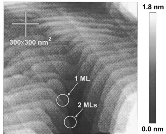
FIG. 2. Shear-force topography image of a GaN epitaxial film grown on a 6H-SiC substrate recorded at  $T=300$  K. Mono- and bilayer steps are indicated by arrows (1 ML and 2 MLs, respectively).
