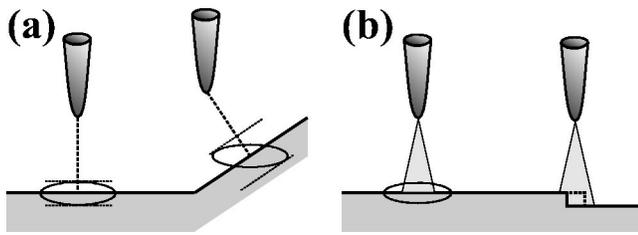
FIG. 3. Schematic illustration of the SAW detection by a SAW-STM: (a) on facets that larger than the tunneling regime, where Eqs. (1) and (2) apply, and (b) at a step of single height, which lies inside the (shaded) tunneling regime.
