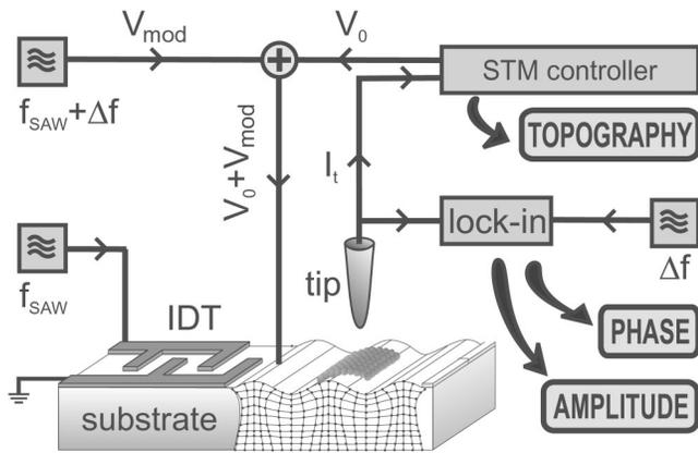
FIG. 1. Experimental setup of the SAW-STM for the measurement of SAW motion. The SAW-induced tunneling current modulation at the frequency  $f_{\text{SAW}}$  is mixed with the modulation of the tunneling voltage ( $f_{\text{SAW}} + \Delta f$ ) at the nonlinear current-distance characteristic of the tunneling gap. A lock-in amplifier extracts the resulting difference frequency signal ( $\Delta f$ ) yielding amplitude and phase of the SAW, which both are recorded in addition to the topography.
