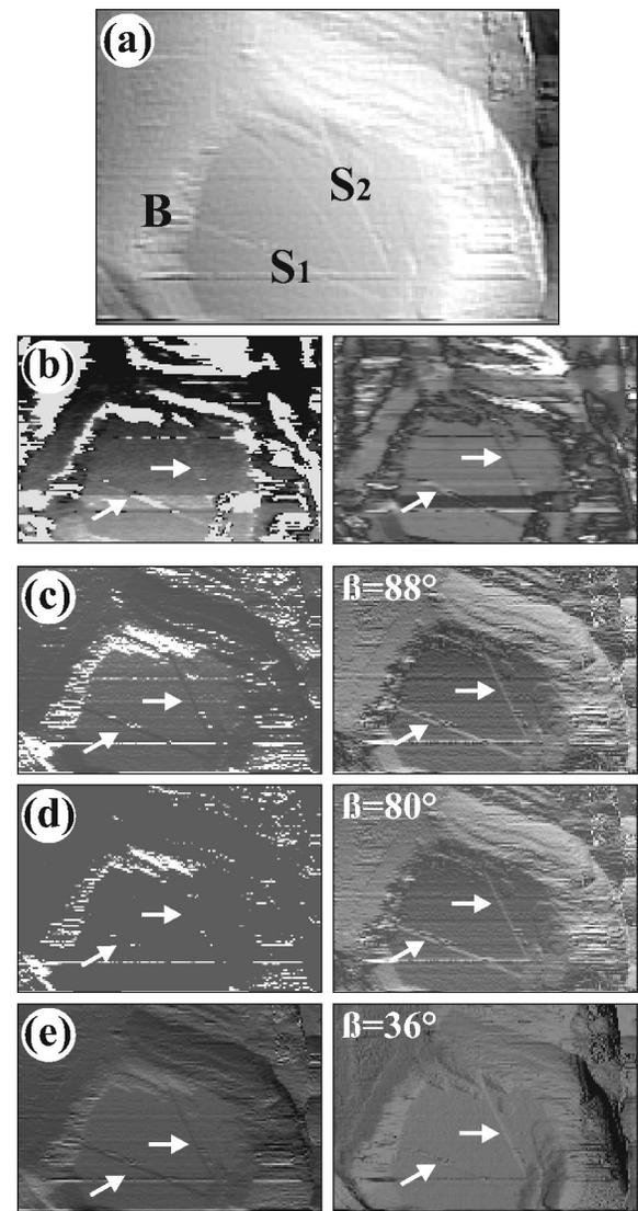
FIG. 2. (a)  $62 \times 42 \text{ nm}^2$  topview of a 100-nm-thick Au film on Y-cut LiNbO<sub>3</sub> as well as (b) phase (left) and amplitude (right) images of a HVP-SAW, all recorded simultaneously with the SAW-STM. (c)–(e) Simulated phase (left) and amplitude images (right) at different angles  $\beta$  of the oscillation ellipse. Good agreement with experiment is achieved with  $\beta = 88^\circ$ .
