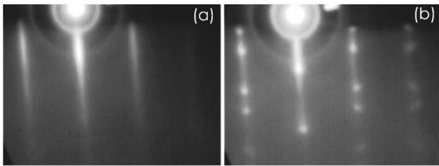
FIG. 1. RHEED pattern along the  $\langle 11\bar{2}0 \rangle$  azimuth of sample B during (a) and after (b) the first 100 nm of deposition.
