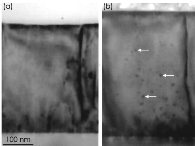
FIG. 2. Bright-field TEM micrographs of (a) sample A and (b) sample B. Note the presence of nm-scale clusters, some of which are highlighted by arrows, in sample B.
