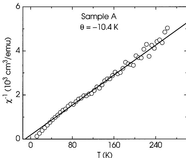
FIG. 5. Inverse of dc susceptibility measured at 100 Oe for sample A as a function of temperature (open circles). The line shows the fit to the data with the Curie–Weiss law [ $\chi = C/(T - \theta)$ ].
