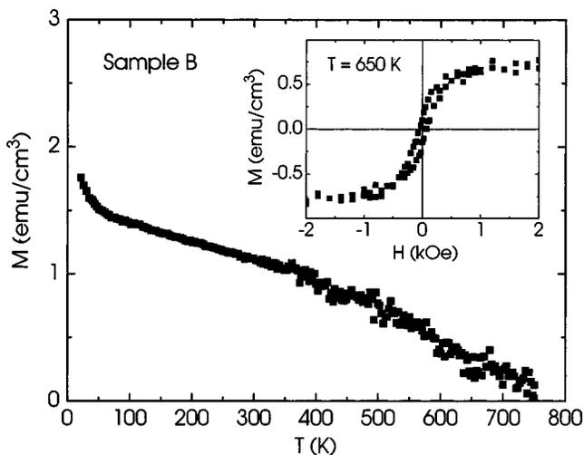
FIG. 4. Temperature dependence of the magnetization of sample B at 50 Oe. The inset shows the magnetization loop of this sample measured at 650 K.
