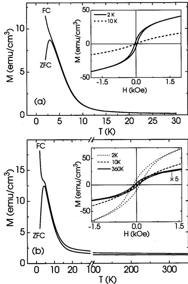
FIG. 3. Temperature dependence of magnetization at field-cooled (FC) and zero-field-cooled (ZFC) conditions for (a) sample A and (b) sample B at a magnetic field of 100 Oe. Hysteresis loops obtained at various temperatures in these samples are shown in the insets of the respective figures.
