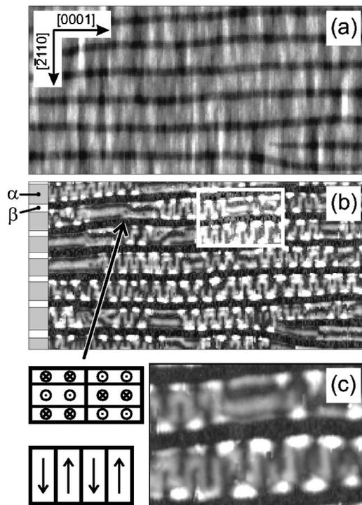
FIG. 1.  $10 \times 5 \mu\text{m}^2$  scans of a 130 nm thick MnAs film at room temperature (21 °C) in (a) noncontact mode that delivers topographical contrast and (b) MFM mode at zero magnetic field. The  $\alpha$  and  $\beta$  stripes are marked. (c) Details of the domain structure [indicated in (b)] along with a schematic picture of the two predominant domain patterns ( $2.5 \times 1.7 \mu\text{m}^2$  scan).
