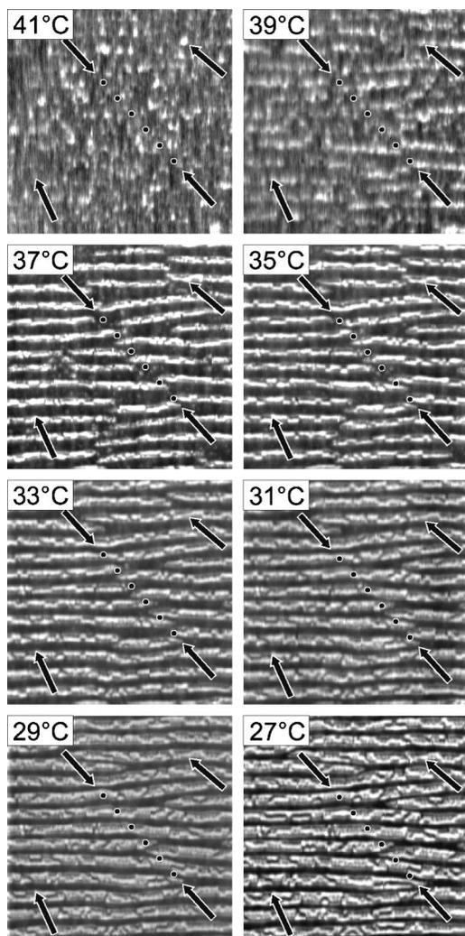
FIG. 2.  $10 \times 10 \mu\text{m}^2$  scan series of MFM images at various temperatures ranging from above  $T_c \approx 40$  down to  $27^\circ\text{C}$ . The arrows and dots mark fixed positions on the sample in order to better visualize changes to the micro-magnetic pattern.
