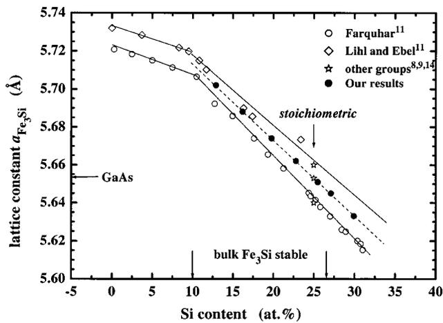
FIG. 3. Dependence of the relaxed lattice constant  $a_{\text{Fe}_3\text{Si}}$  on the Si content for the  $\text{Fe}_3\text{Si}$  phase. The solid lines are guides for the eye. The dashed line gives a mean value in the range of 10 to 30 at. % Si. The solid dots are taken from the results shown in Fig. 1. Note that a larger value of  $a_{\text{Fe}_3\text{Si}}$  belongs to a lower  $T_{\text{Si}}$  in Fig. 1.
