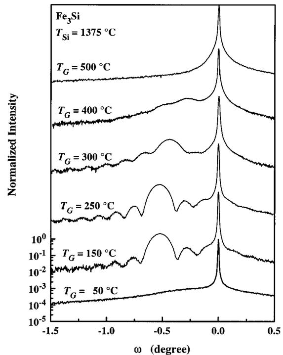
FIG. 2. Semi-logarithmic plots of the normalized intensity of DCXRD rocking curves for various  $\text{Fe}_3\text{Si}/\text{GaAs}(001)$  layers grown at a fixed  $T_{\text{Si}}$  of  $1375^\circ\text{C}$  dependent on the growth temperature  $T_G$ . The curves are normalized to the  $\text{GaAs}(004)$  reflection of the substrate. The rocking curves are shifted for clarity.
