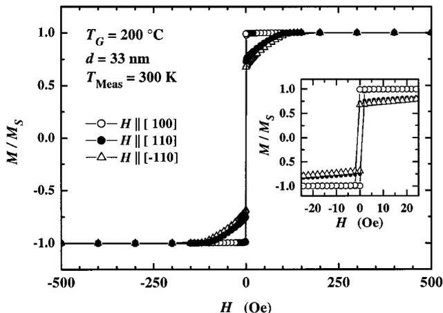
FIG. 4. Hysteresis curves measured at room temperature for a 33 nm  $\text{Fe}_3\text{Si}/\text{GaAs}(001)$  layer with the magnetic field  $H$  applied in the film plane along various crystallographic orientations. The magnetization  $M$  is normalized to the saturation magnetization  $M_S$ . The inset shows the hysteresis at very low fields.
