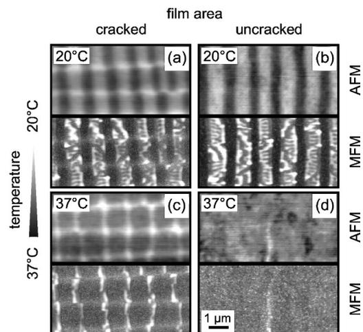
FIG. 3. AFM (upper half) and MFM (lower half) scans of a cracked (left column) and an uncracked (right column) surface area, as described in Fig. 1. The upper row images were taken at  $20^\circ\text{C}$  and the lower row images at  $37^\circ\text{C}$ ; that is, close to the phase transition temperature.
