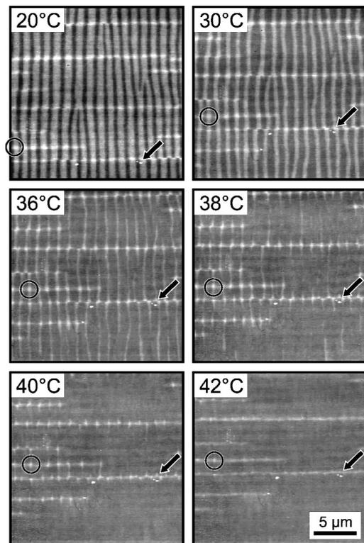
FIG. 2.  $20 \times 20 \mu\text{m}^2$  topography scans. Evolution of the  $\alpha$ -/ $\beta$ -MnAs stripe structure upon heating from 20 to  $42^\circ\text{C}$ . With increasing temperature, the amount of  $\alpha$ -MnAs decreases, as can be seen by the decreasing width and length of the bright stripes. Above  $40^\circ\text{C}$ , almost all the entire  $\alpha$ -phase has vanished, except in the vicinity of the cracks.
