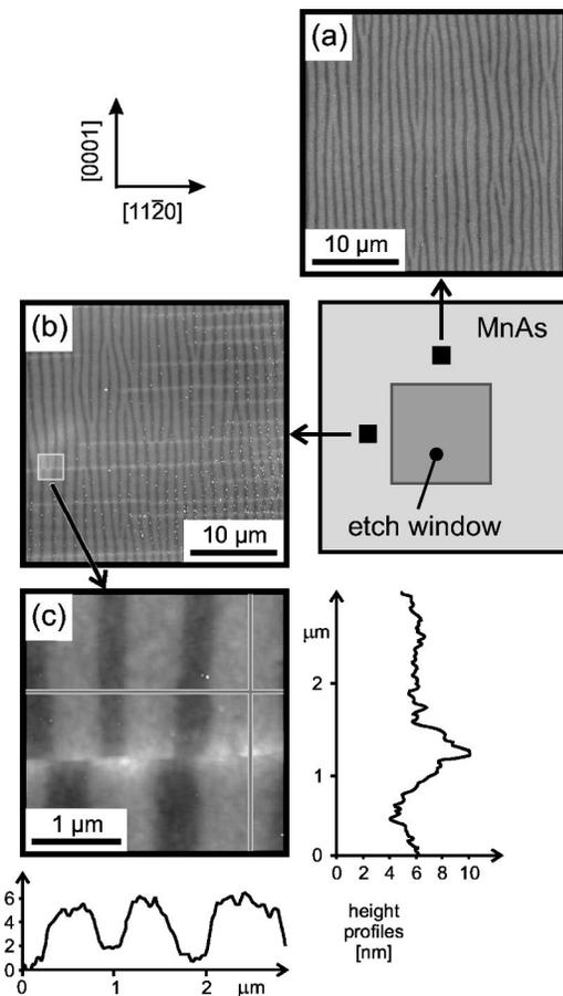
FIG. 1.  $30 \times 30 \mu\text{m}^2$  AFM topography images of the un-cracked (a) and cracked (b) MnAs surface. The 215-nm-thick MnAs film was wet etched through a window (see dark gray area) leading to a regular row of cracks running in the  $[11\bar{2}0]$  direction. The zoom of the cracked surface area (c) shows a shift of the periodic  $\alpha$ -/ $\beta$ -MnAs stripe structure across the crack. The line scan across the crack reveals that MnAs is piling up upon crack formation.
